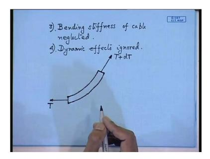
Now, number 3 is bending stiffness of cable line now we are making static analysis. So, right at the top you write static analysis. So, these are not to be confused with quasi static or dynamic analysis. So, you do not make any dynamic effects dynamic effects ignored. So, before we proceed in the calculation that is with the free body diagram. So, next I will try to draw the free body diagram. So, you make these assumptions. Now, let us take a portion of the chain cable say at this point.
