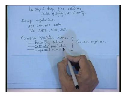
Now after this painting and corrosion plans corrosion protection plans. Now rather you have to specify the corrosion. So, here you have to convince or you have to tell your plan your painting scheme. What paint protection you are giving? Catholic protection by means of sacrificial anodes if you have and sometimes they may give; I do not know anything; I am not a corrosion engineer. So, they call impressed current.
