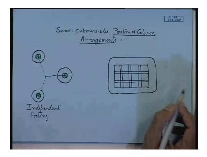
Now, the important thing that we will discuss is pontoon and column arrangements, so how we arrange the pontoons and column in your semi submersible. So, this is a wider issue, now the overriding principle that governs is reduction in the weight force and motions. Now, if you want to do that, there are number of positive and negative points which you come across.
