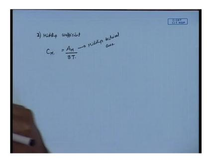
So, this is known as the block coefficient C B given by del divided by LBT. Then, there is a first coefficient of form. These, as I told you, these things are coefficient of form. First is block coefficient; then, next one is something known as mid-ship coefficient; this is known as mid-ship coefficient. Mid-ship coefficient is defined as A M. It is usually written as C M. It is known as A M divided by B into T.
