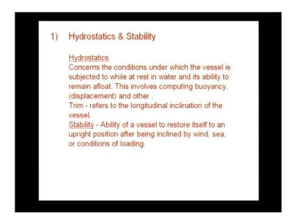
So, these conditions, we will be dealing with. These conditions are studied under the concepts of stability and hydrostatics. Then finally, the main thing that is how the vessel is able to restore itself to an upright position after being inclined by wind, sea or conditions of loading.
