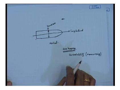
So, if you have a ship like this, then this direction, we usually call it as longitudinal and this direction we call it as transverse and the third one, of course, is known as the vertical. So, we have three directions for our ship. We have the longitudinal, transverse and vertical directions.
