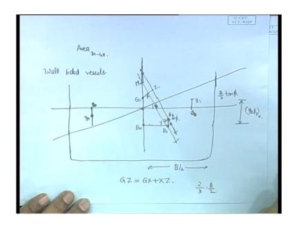
So, I am talk about this g 0 g 1. It is the shift in the center of gravity, center of, either of those centers of gravity of the wedge or the center of volume of the wedge, either way you can look at it. So, this volume, one volume goes in, one volume comes out. So, this volume goes in, this volume comes out; as a result of which this wedge is coming out, this wedge is going in. Again, as a result of which one volume is it is like a one volume shifted from one side to another side.
