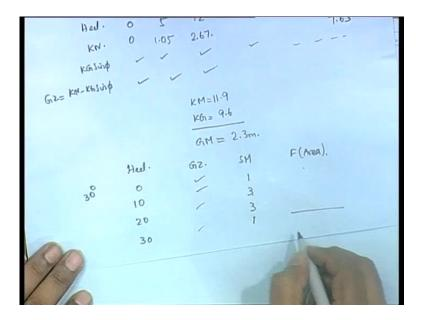
So, you have to find the area. So, that is like this only, heel, G Z, you write the Simpson's multiplier then function of area; 0, 10, 20, 30, so you find the area up to 30 degrees. You have to in fact to do two things; you have to find the area up to 30 degrees then you have to find the area up to 40 degrees, and you have to find area between 30 and 40 degrees both, all three things you have to find.
