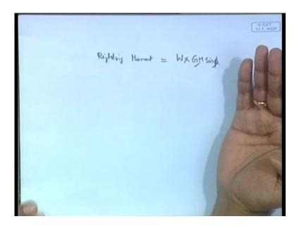
The righting moment is given by the weight of the ship into the GM sine phi. You asked the righting moment at 1 degree heel, so phi is known, GM we have just calculated if you use the one for the intact condition you get for intact righting moment and the other one you get the damaged righting moment. Now, as you can think by intuition itself, you will see that when always you have bilging the righting moment decreases as a result of bilging.
