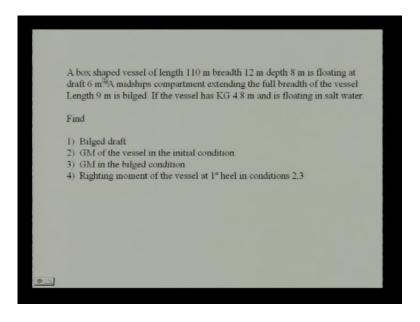
For instance this one says that there is a box shaped vessel, which has a length of 110 meters, it has a breadth of 12 meters, and depth of 8 meters is floating at a draft of 6 meters. The mid ship compartment extending the full breadth of vessel of length 9 meters, so the length of the compartment is 9 meters and it is extending the full breadth of the vessel is bilged.
