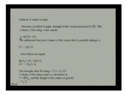
Now, in this case the problem is slightly simpler infact that is you have the ship, you are adding a weight to the ship that is the problem. You are adding the water to the ship and the ship sinks, so there is an increase in draft. In this case, let us assume that the increase in drafts is delta T and then, you can see that what the volume of flooded water is. So, that is what we just said the volume of flooded water if you look here is v is equal to l into B.
