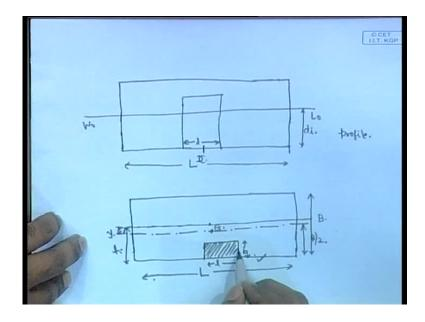
You will get h to be L into B into B by 2 and moment is means here, you have a L into B this is the whole area and into the position of it is center of gravity which is B by 2. So, L into B into B by 2 minus – a small area is gone here, this is of small 1, it is of breadth small b and it is centroid is at a distance small b by 2.
