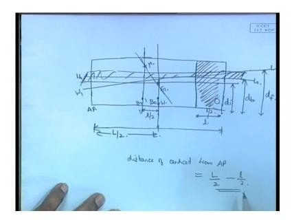
In this case, let us consider the ship in the box, so you have the box shape vessel, so one compartment like this in the front part of the ship gets flooded. Let us say that there is a hole here, this compartment gets flooded here, this is of length small l, the total length of the ship is capital L, so this compartment gets flooded.
