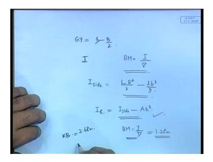
Remember, the main purpose of our work is to find tan phi which is equal to given by GY by YM, this explain to be the equation for tan phi. First thing we need to calculate is GY which is equal to h minus B by 2, I have already described it I need to describe it again h minus B by 2.
