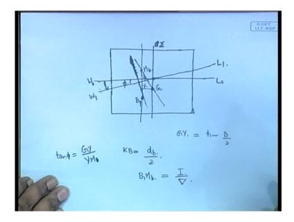
From that you will get BM equal to I by del then once, you have that let us look at this figure, you see that if it is tilted through an angle phi, from this you can directly read that tan phi is equal to GY divided by YM. In this case, GY we have already calculated it is equal to h minus B by 2, which is the distance between the G and that vertical position of M or the position of the projection of M, so that gives you GY divided by YM.
