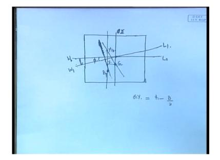
Now, just like that if you draw, this is the box shaped vessel, now for this we are drawing the. So, this is the section, let us consider this to be the initial water line and the final water line. Initially, the ship is at G, it is at midship section. So, this is G; somewhere you have G, where the weight of the ship is acting.
