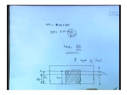
Just like I explain the previous problem it is come something like this. So, you have the center line and in this case a midships compartment somewhere here a region is flooded. The breadth of the ship initially is 9 meter - this is 9 meter - and his breadth of 6 meters. One compartment like this of 6 meters, so this is of breadth 6 meters, so out of the 9 meters 6 meters length, this region is flooded.
