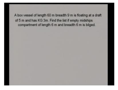
Now, we will look at one problem; suppose, you are told that there is a box shaped vessel of length 60 meters, breadth 9 meters and it is floating at a draft of 5 meters and it has a K G of 3 meters. You are asked to find the list if a midships compartment of length 6
