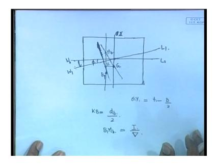
Then other things we need are one KB, we have to find the final KB of the ship. We always say that KB is the vertical distance of the center of the buoyancy from the keel, now that distance is always measured as half the draft, whatever is the draft. So, it is d b divided by 2 this will give you the KB. Another thing we need to calculate is BM, in this case BM which is equal to defined as I by v or I by del - I by del that is the metacentric radius is defined as v 1 M b is equal to I by del.
