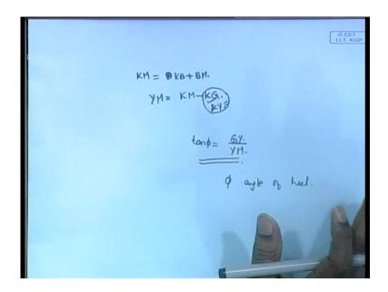
Once, you have that you get KM is equal to KB plus BM, YM is equal to KM minus KG. Just look at this figure YM - why is it so, because remember this will be the keel. So, if you are looking at the vertical distances KM; this vertical distance is the same as this vertical distance. So, this is KG, this is also equal to KG, KG YG or KY is equal to KG. This KG is actually equal to Y KY which is equal to KG because of this you can get this expression.
