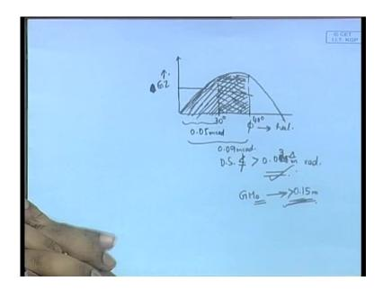
And you have the GZ curve and let us suppose that you have a curve like this so this is what we call as the and delta into GZ if it is instead of GZ if it is delta into GZ this curve becomes a the area under this curve becomes the dynamical stability.
