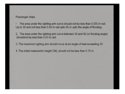
We will go into some rules that are very important, the first of which is the set of rules dealing with passenger ships; now some of as I have said before its always like this so you have the phi curve that is the heel.
