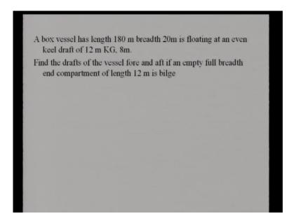
So, this change in trim will be given by, W into I by MCTC. So what we need to know is the weight of the ship and the distance between the center of gravity and the center of floatation. For instance, you might end up with the problem like this.
