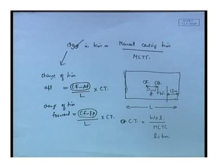
Now what this says is that in this problem, if you look here a compartment which is of length compartment of length 12 meters, what it says is that compartment of length 12 meters gets flooded here. Now if you remember the previous class we saw that this distance between the center of floatation and the center of gravity will be equal to this length divided by 2.
