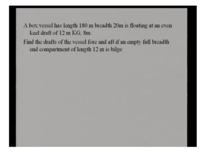
So, what is a easiest way to do this is you can see where the load is added for instance in this problem. You can see that the ship is bilged in the forward direction; it is given in the full forward. In this problem it is given though it is given here, but the problem is that the ship is bilged fully in the forward compartment.
