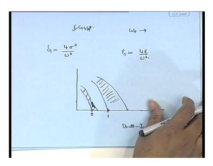
Now, we have this epsilon cos omega t. So, I just want you to know, what are the two types of frequencies we talk about here? One is the natural frequency of heel, if this equation, I mean in this case, this does not represent the heel motion, it is x double dot; so, it is not heel motion; it is represents the natural frequency of whatever translatory motion. We are discussing here the natural frequency of that motion of the ship natural frequency.
