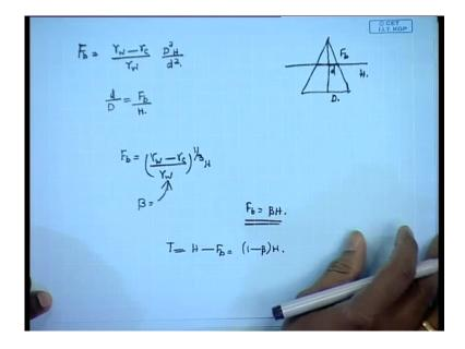
So, this is the Archimedes principle. This is the first equation that we have. So, from this we get F b is equal to - just by doing some arithmetic on the previous equation by gamma w into D square H by d square. Now, if you apply similarity theorem, so this how we have here. This is the water line, so we have here F b; we have here total distance H, d, D, this distance and this distance.
