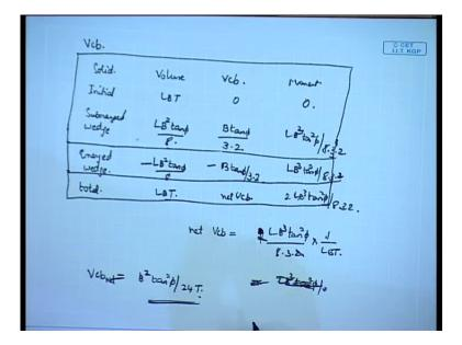
Now, L is cancelled, B square tan phi by 12 into T. So, B square tan phi by 12 into T will give you the net tcb of the whole system, after it submerges and emerges. Now, similarly, we need to find the vertical center of the buoyancy. This is again following the same procedure. This is to find the vertical center of the buoyancy, what we need to do is again solid, volume, vcb of that portion and the moment.
