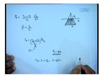
Then draft T is equal to H minus F b is equal to 1 minus beta into H that is the draft of the cone. Then, you will have K B of the cone - K B of the cone is given by (Refer Slide Time: 08:40). This gives you the diameter; this gives the center of the buoyancy. What you really have here is the centroid of this; what we want is the centroid of this region. So, the centroid of that is given by this formula D plus 2 d by D plus d. Now, this is the
