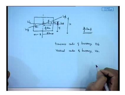
Now, let us consider another problem; that is, there is a parallello pipette - pipette barge - parallello pipette barge, which means this is a rectangle, all such barges are also called as box shape barges. It is like this, so your cross section is a rectangle and anywhere it cross the whole thing is a parallel pipette barge; means whole thing is a box, it is just a rectangular box.
