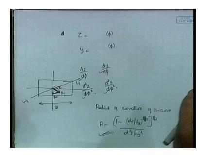
I will show this figure; may be this figure, it will help; that is, this is B. When it was vertical, this distance was B, but when it is tilted like this, this distance is not B anymore; it is slightly more than B. Then, B by cos phi it just it [jus/just] is just the algebra; it gives to B cos phi cube by 12 divided by LBT.
