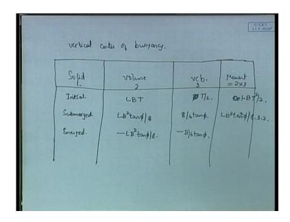
Now, first you have the whole initial width, before it is the whole, before the whole thing is inclined. So, the volume is again LBT vertical center of buoyancy that is 0 0. Then, submerged, the volume is again the same. This is the volume that is submerged. We have done it last time. In the previous table, we did this by 8 and this we just the what is this v v c b of that wedge; you said that is b by 6 tan phi.
