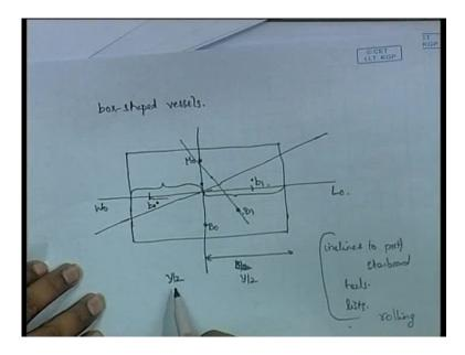
The volume of the wedge is v and centroid is moving from b 0 to b 1. b 0 to b 1 is equal to 2 twice this same as what we did last time, just before - 2 by 3 into y by 2 is equal to 2 by 3 y, where, in this derivation we are just putting this to be y by 2 and this is y by 2. This distance is - Because we are deriving something, let us put it as y - this is y by 2 and this is y by 2.
