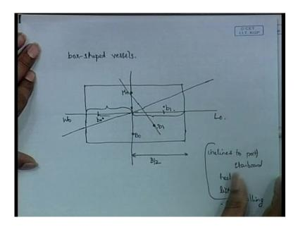
What is b 0 b 1? What is this distance? We know that this distance is 2 by 3 of this whole distance that is, the center of buoyancy of a triangle. And this distance is 2 by 3 of this whole distance. So, this 2 by 3 plus this 2 by 3 will give you the distance between b 0 and b 1.
