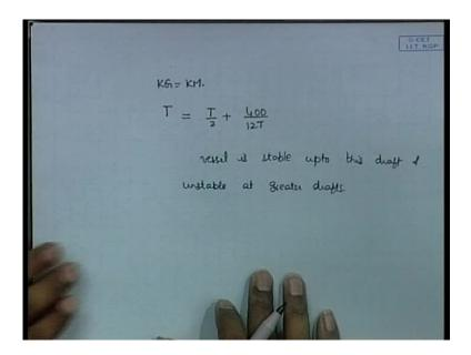
So, GM is equal to 0 and if GM is equal to 0, then KG is equal to KM. You already have what KG is? KG is given to be T and KM; you have calculated using that formula, so that is T by 2 plus 400 by 12T. Just before we did that and now we will just solve the equation.
