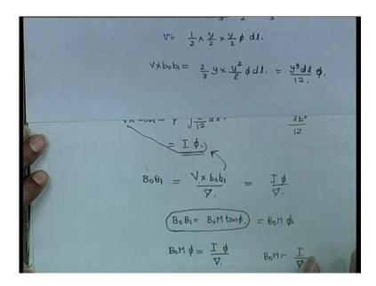
Therefore, what do you get? B 0 M phi equals I phi by del, which implies that B0M is equal to I by del. This shows that this is true only for a box-shaped body. You could probably use this method to really derive the general expression, if you want. It is not that difficult, because the only thing that will change is probably the volume which you cannot define so specifically; but, if you work on this you might be able to do it.
