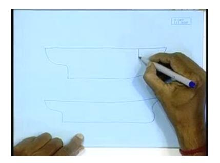
Today we will start with the ford end and after end construction. To some extent we have talked about it in some of our previous lectures. I mean as you can see the name, ford end construction, so it is written like this end or also it is written as fore end. That means the fore end of the hull, this part only. What is the great difference between these two hulls?
