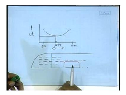
So spacing between the longitudinals also will be equal to that frame spacing. If you are providing a centerline girder, if you are providing a girder here, suppose I have hatch opening here then this particular longitudinal is replaced by a hatch side girder.
