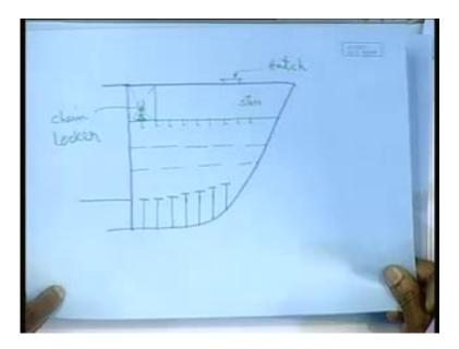
We have the chain locker and then the stringer, two stringers we have shown. It is nothing but a member like this. In the profile view along the length, along the side shell, that angle section is going like this. If I take a section here, along this, this section is this one, so stringer is coming here in this fashion. (Refer Slide Time: 46:13)
