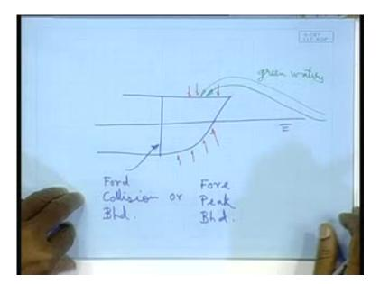
The deck plating means you have the, suppose I am just drawing the ford part of the ship, this is your water surface. In a bad whether there can be, it can the waves may become too high and come and hit the deck. So you need additional strengthening at the deck, to
