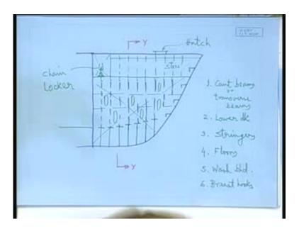
So you needs to be stiffened. They are referred to as breast hooks. That is how the name - breast hooks, they are referred to as breast hooks. So well, that is what is the little elaborate sort of construction arrangement for the ford end. The whole idea is to make it more strong, locally more strong; by floors, by stringers, by breast hooks, centerline bulkhead and then well the deck beams or cant beams.
