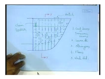
So what we can see? To make the ford end strong what we have put is that all these structural members we have taken to the course to. What we have taken? Well in the deck the cant beams or transverse beams, it can be or transverse beams. Here we have shown the example of cant beams. Cant beam is somewhere in between longitudinal and transverse, is going radial. Then second what we are doing? Well by virtue by providing another lower deck that adds to the strength.
