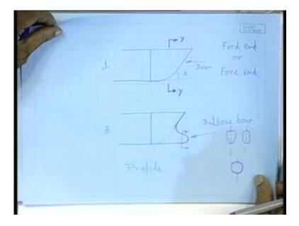
So as we go for stiffening arrangement, then we see that a somewhat little extra care is given to this ford end constructions. Though we have talked about that, if is the primary strength considerations are essentially because of the longitudinal bending.
