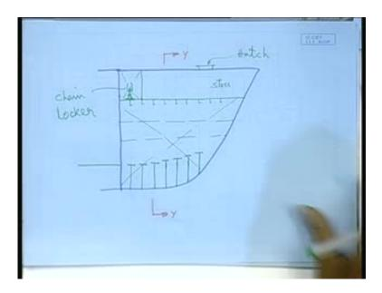
Well that plate may have opening here, lightening hole. Then what about these spaces? What happens is depending on the requirement etcetera one can have even a central line wash bulkhead. This I have drawn, that means there is a central line bulkhead, a plate here in the central line.
