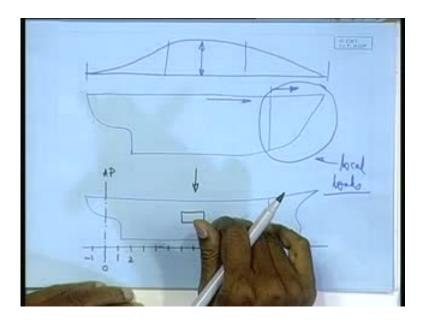
So from there you choose what is the but the basic philosophy is this in the behind, that you choose what should be the frame spacing. Once the frame spacing is done what does that mean? That means the spacing between these lines I have drawn, they are basically say 800 millimeter. That means at every 800 millimeter there will be a stiffener or every multiple of 800 there will be a stiffener. So if say the side shell is transversely stiffened I will have every frame position a transverse frame.
