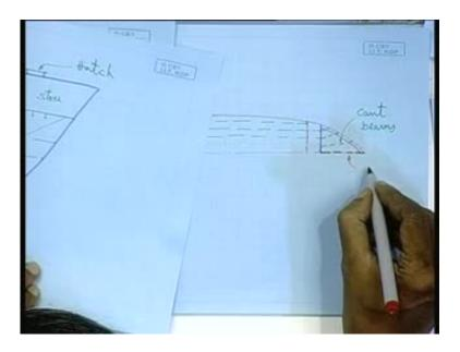
That means that will be visible well, this one here the red dotted line, this is my central line bulkhead. That means provided a central line. By central line bulkhead means a full plate, but obviously the plate we are keeping it, that will have its stiffeners connecting from the beams to the floors.
