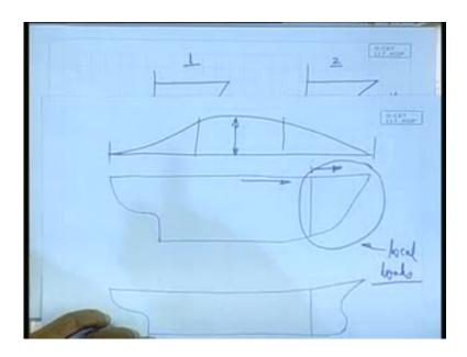
So in any case what we like to highlight is, that means the ford end of the ship is subjected to primarily local loads, local loads of various kinds. One is due to the ship motions of heave or slamming, that is, the underwater hull will get affected because of that, another is as we have said that the deck plating.
