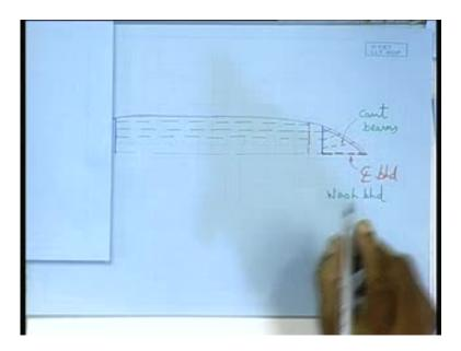
Because it is a longitudinal member. Then you have in this those well, in the same fashion those big openings to keep it in a lighter condition. as well as right This is a longitudinal member here. This one this is a central line bulkhead. It is also referred to as wash bulkhead, because this bulkhead is not the one we have talked about, transverse sub division bulkhead.
