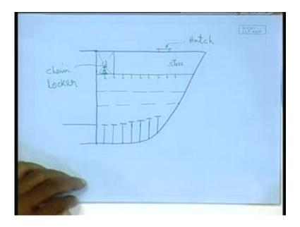
In addition to that, what we will have here is, at every frame location you will have the plate floors. Obviously, here you do not have the concept of double bottom. In the rest part of the ship there was double bottom.
