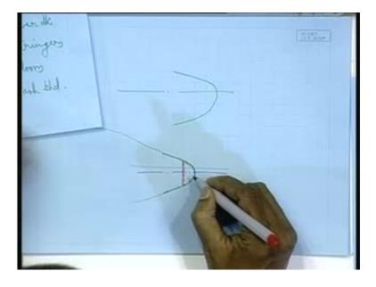
This is a small plate welded to the bow. That the bow plate only in the, where it has been bent. The entire bow plate is coming right from here, this whole plate but I am stiffening only a small part. How small it should be or how big it should be, that is a matter of so called design. So these stiffeners they are in addition, you see all these again in addition to that, because this forward nose, that is a nose of the ship that will hit maximum.
