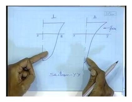
Suppose this is my y y. About this y y the sections are taken, obviously of two different forms. So what we can see here is that this particular is having a much larger flare. Both are suppose they are having the water line here. In this we see that it is having a must more flare, this is what is referred to as flare.
