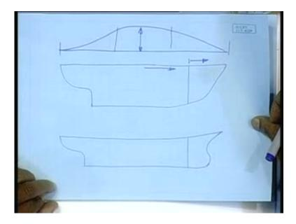
Because of the longitudinal bending, the longitudinal bending movement is somewhat like this. So we see that around the mid length of the vessel I have maximum bending movement right. This is my bending movement curve, so as we go forward or aft the bending movement is zero. The load coming due to the bending movement or the stresses generating due to bending movement in the ford end is gradually going down, it is lower.
