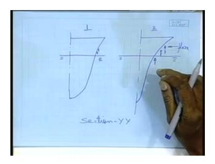
That means there it is no more the case of the stresses due to bending moment, but it is the local loading which comes into play, local loading takes over. So in these two forms as you can see if both the vessels are plying and imagine it meets a somewhat rough weather and the vessel starts heaving, heaving means it goes vertically up and down.
