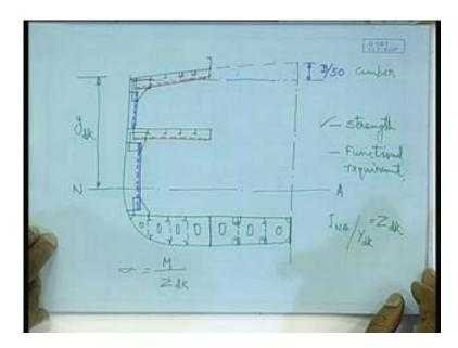
So, the spacing between the transverse would be 3 to 4 frame space, 3 to 4 frame space so this transverses will provide the support, so again the same thing here, you will have this small this so called openings, like in the floor you had like in the same connections, here the intersection of the inner bottom longitudinal and the floor plate or the intersection of the bottom longitudinal and the floor plate, whatever is the detail we have already discussed about it will be same here also.
