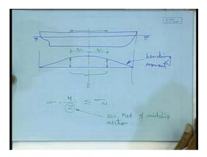
So, here I have shown, a zone of one-fourth of the length of the ship, aft as well as onefourth forward, because what we see that, in this region the bending moment appears to be maximum within this zone within this zone of one-fourth the length of the vessel in the aft one-fourth in the forward, we have a bending moment distribution which is on the very higher side.
