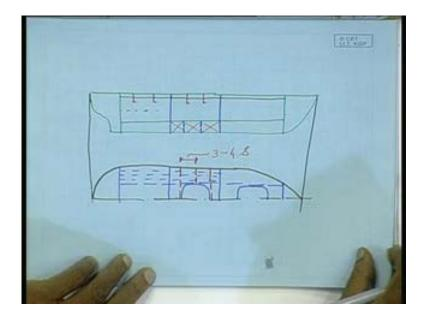
Side girders are generally made intercostals that means between two plate floor the side girder continuous, what is that mean? That means that would be visible in a longitudinal section.
