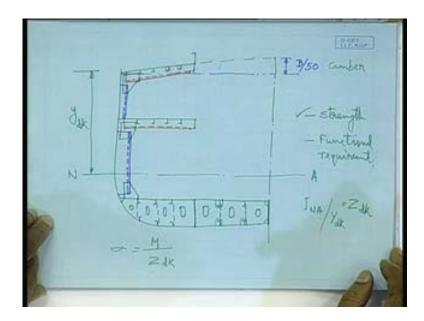
So, finding out the neutral axis and finding out the section modulus of this, how do we get that well? We get from to that will take only those longitudinal members obviously, this deck transverse, side shell frames will not contribute naturally, they are not contributing towards longitudinal strengths, so there sectional modulus does not come into picture.
