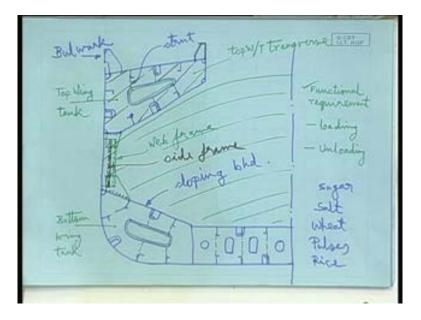
Now, along with bulk carrier we have talked about the OBO carrier;OBO is Ore and Bulk Oil - I mean -that is how it is named.In this particular vessel we had been taking aboutcargos likesugar, salt, pulses, wheat, rice all in bulk - in lose. (Refer Slide Time: 33:59)
