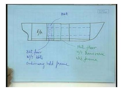
Bulk carrier side shell is also transversely stiffened and the bracketing arrangementgoes something like this, the side shell. So, that is how we have the arrangement midship section arrangement for them. This is the transverses here, this top wing tank transverse this what I have drawn is a plate - this is a transverse.
