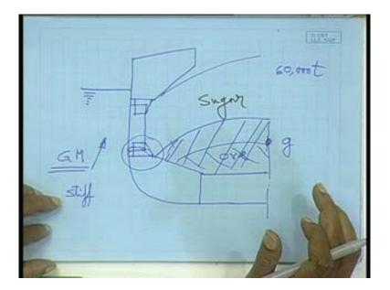
What weight?Does not matter,thing is that I have my load water line here defined that means, beyond that I cannot load.So, I go on loading and when I find that it has touched the load water line I stop my loading. So, it has taken in suppose, the bulk carrier is designed for carriage of 60000 tons of cargo,when it touches this line means I have achieved those60000 tons.
