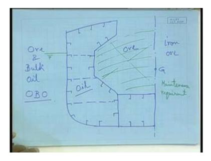
That is how the structure arrangement will be done that means, so what we see that the structural arrangements are done based on functional requirements.Second is first and foremost well structural arrangement is this one on the criteria of strength, also in functional thing.
