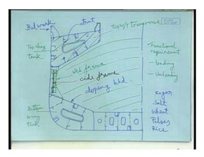
We will have these transverses they are in one plane, the top wing tank transverse. In the same plane you have a side frame, in the same plane the bottom wing tank transverse, same plane plate floor.
