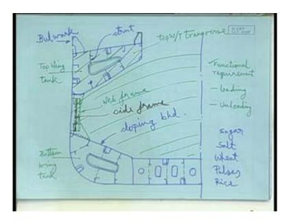
This is what thestructural arrangement - midship section structural arrangement for the bulk carrier. Obviously, on the deck you have here is what is referred to as a bulwark. Here, you the hatch coaming, this is what is these are all you will have in all vessels.
