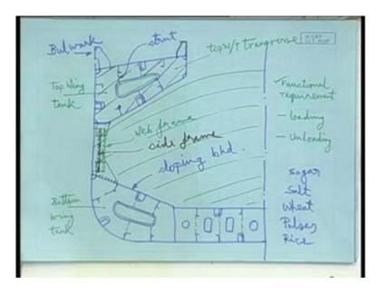
Thereby, we come to the section shape like this. What happens in that case is here we have the cargo loaded like this, the entire cargo is there. So, while loading automatically this corner is taken care of and while unloading again this corner is taken care of, it has been given a right amount of slope such that you will slightdownand thereby the form comes.
