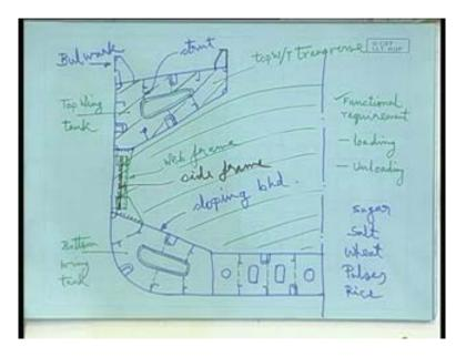
What happens in case of a bulk carrier?Bulk carrier, as the name you see that it carries cargo in bulks. It has a loading pattern as well as I will have to think of how unloading will be done. Loading and unloading are two important aspects in cargobecause, if we have a mechanism by which I can load the cargo faster as well as, unload the cargo faster
