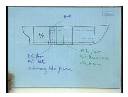
What I am saying is like this.Here, I have a floor all these transverse members, in green I am drawing, this is my plate floor.In the same plane you have the bottom wing tank transverse, in the same plane we have the web frame top wing tank transverse.
