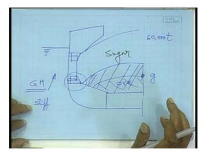
In one voyage I can carry ore, in the return voyage I can carry oil; some kind of oil some kind of liquid. That is the advantage otherwise, it would have been a bulk carrier then if I carry iron ore in the return voyage I will have to carry either coal or equivalent some such product nothing else can be carried not even oilbecause they will contaminate.
