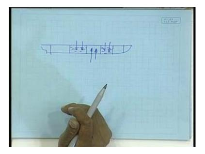
What would be the solution?One solution could bealternate hole.Then, I can fill to a much greater depth, so then that shearing problem will come.If alternate holes are filled up then what is happeningphysically it would look something like this.
