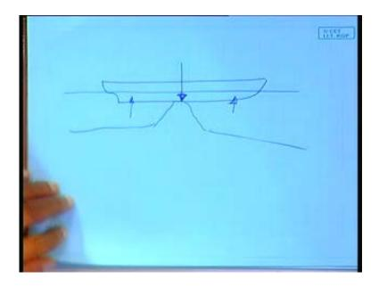
Grounding of a vessel means you have... so, what is happening when it is floating. You have huge buoyancy working here and where it has got grounded, the entire load works here.
