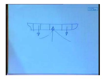
Sorry just opposite way I have shown, there buoyancy is working well the moment it gets grounded, the moment it has got grounded means; the entire load is working downwards. So, the reaction force, total reaction force, here you have the engine, also you have the holes are full.
