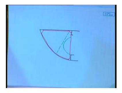
Longitudinal of the inner bottom plating and the longitudinal the bottom shell plating. So, it is connecting and here you can see something not very clear that is nothing but again a stiffener because your this thing can be this plate is getting under completion this bracket may buckle.
