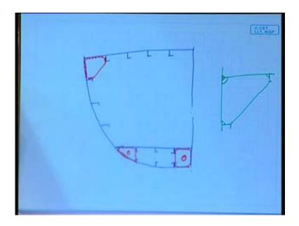
So, load path is being implemented basically whatever load is coming on the deck is getting transmitted to the side shell. So, it is helping in the transmission process. You assume this bracket is not there. So, as if the deck, the entire load is being transmitted through this joint at the corner. Only then this joint of the deck to the side shell. So, what would have happen, this is the side shells, this deck plate it is welded here.
