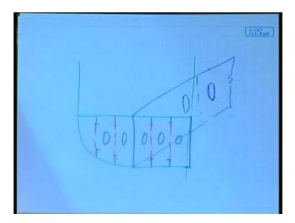
A side girder it is. This is a floor, this is a side girder means you have the... See your double bottom and then you have longitudinals and inner bottom longitudinals. You have a side girder, this side girder this side. So, the floor is there.
