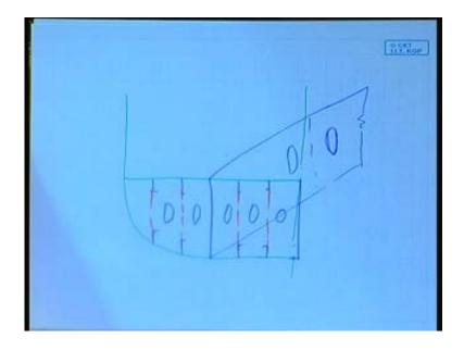
Here you have the center girder. So, this plate is the floor, the transverse floor with the struts. The struts you can see there. The struts welded to the inner bottom plating as well as to the bottom plating and you have this openings for the floor and they are in the perpendicular to this is a side girder; this vertical line this is going along the length.
