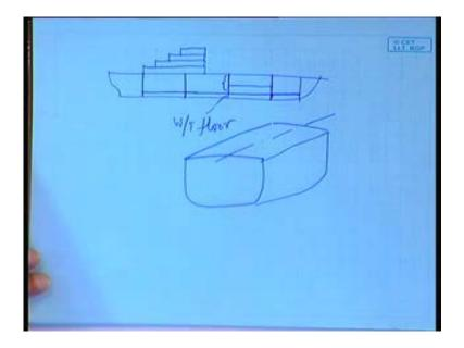
Because you have the ships well as you, the well the double bottom is there and the ship is divided in various compartments water tight compartments. That means, each of these compartments are individually water tight or in other words any damage in any compartment, the flooding whatever will take place, will remain confine to that compartment. That will not spread to the other compartments; that means what, these bulkheads should be able to withstand that force.
