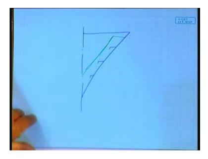
The fore forward sections if we draw, the forward sections have become like this sharply v type. So, this is my one of the I mean in the forward section where I have the side shell longitudinally stiffened.
