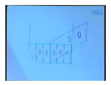
Generally side girder is not a water tight girder, a center girder is generally water tight why because then you have a port side tank a starboard side tank.
