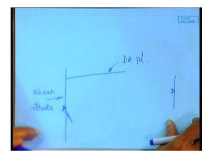
Again get back to this first slide. Well here I thought there will be one this simple things may be of interest. Here if you see a little close up of the construction, it is always like this, the deck this is my deck plating. This is the side shell plating, this part of the side shell is referred to as shear strake. This particular plate is has a special significance.
