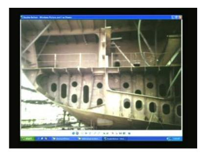
So, within that this plate has to be stiffened. So, you just provide a at certain angle a stiffener. Just to and the stiffener is also it has the same function as that of a what do you called strut basically a strut. So, well may be next one let us see.
