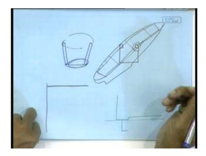
So, bulkheads are there. So, in the process what happens, if the bulkheads are there like here I have drawn in red. So, this longitudinals in the box girder in that case will be running from one bulkhead to another bulkhead. So, this again becomes a quite a huge span. So, again from the same logic, we will have transverses in between like we had the deck transverses in the general cargo carrier or bulk carrier.
