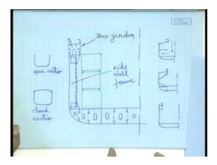
Rightly pointed out that this side plate or the deck plate as well as this side shell plate are stiffened by stiffeners; longitudinal stiffeners longitudinals whereas this bottom plate is not stiffened as such, I mean we are not seeing any stiffener here. What is happening; this is getting stiffened from below by this bracket because a huge bracket is being welded at every frame position.
