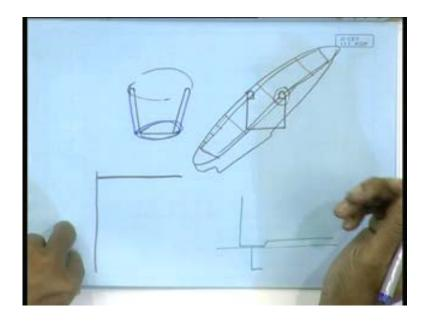
That means, the container edges there is a small actually the container edge is something like this. So, it should sit suppose on the deck and there should be a stiffener there.
