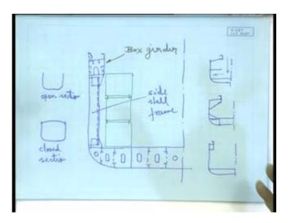
So, the arrangement should be done in keeping that in mind that it should the load path should be there proper load path; that means, it should sit on some stiffener below.
