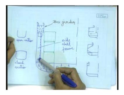
And for we have talked about we have containerized the cargo because of easy loading and unloading. So, if you have to do that we will have to have a mid-ship section something like a open section means fully open. Till now all the vessels we have seen, if I just make a comparison here, we can say the all the other vessels had a hatch opening like this; be it a general cargo carrier or a bulk carrier.
