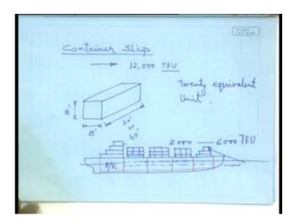
So, that is what the basis of container ship is. So, in the process what happens, we have seen general cargo carrier, bulk carrier, we have talked about carrying capacity in terms of tons, dead weight; how much dead weight. How much cargo it can carry in terms of tons 12000 tons, 60000 ton like that. Whereas in container, we talk in terms of T E U 20 equivalent unit.
