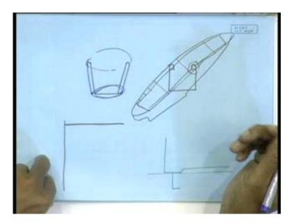
If I keep the edges without any stiffening, it does not have any torsional stiffness. Just to provide stiffening this is bent like this. Those plastic tumblers, domestic tumblers that gives you the strength. So, here imagine the case, instead of I mean we are just simplifying it trying to draw equivalence. This and instead of turning out side say I turn inside I also have the same stiffness.
