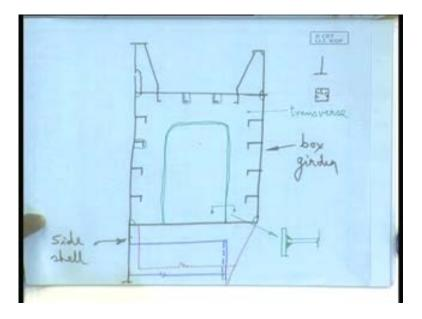
How heavily what basically is done? If I just enlarge that part of the box girder, it is nothing but such enlarge section of the box girder. This is your box girder. This is the side shell plate. Here you have as usual the Bul work and or railing whatever. You have this hatch opening here; this is the hatch coming. So, only this much is my deck then rest is full open. So, what is done is this is your side shell. We will just take a look how it is done in other vessels. (Refer Slide Time: 19:00)
