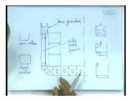
Side shell is transversely stiffened with heavy bracketing at both the ends and bottom part well a double bottom like in any other vessel. So, with this one can go up to a certain size. Then it was found that when we are talking about 9000 T E U, 10000 T E U bigger and still bigger vessels, then it was suggested to go in for a construction which will provide you the required torsional strength.
