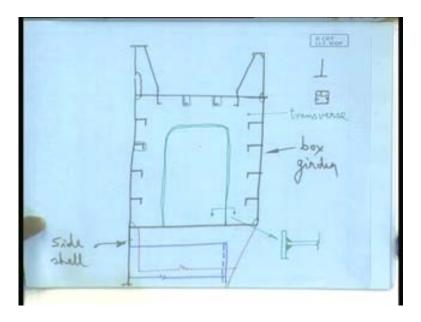
So, that it is may be this is side shell going and this is a part of the transverse frame which is now which will be suitably bracketed; that red line is the part of the bracket is being shown, the blue line part of the side shell frame is being shown as you can see here.
