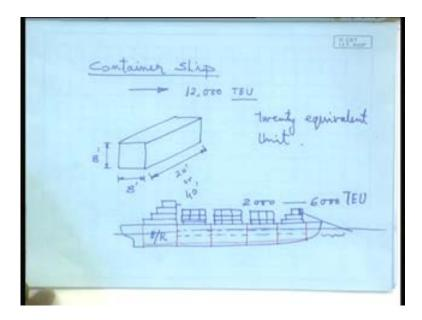
Well what is a container ship basically? As the name, you can see that it carries containers. Containers are somewhat of this type, somewhat means, they are essentially a rectangular container. As you can see, the dimensions are they have a cross section of 8 feet by 8 feet, and length either 20 or 40 feet, they are in feet; this is the universal standard, means all the containers which are used in the container ships, they will be either 20 feet long or 40 feet long.
