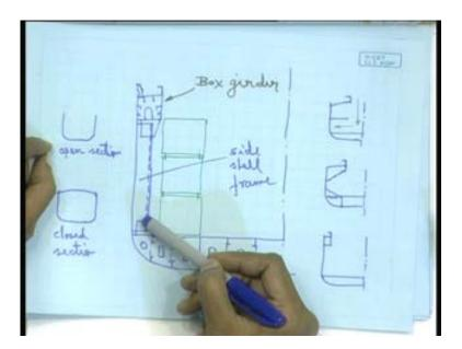
(()) Yes bottom side we have not provided because you see the construction. In the bottom side at every frame space this frames are coming and they are bracketed to the bottom plate. So, bottom plate is stiffened by these brackets.
