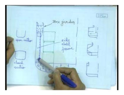
Well. So, that is what is about the container ship. So, we can see that here if it is a box girder kind of arrangement, then we take a combination of longitudinal framing system and transverse framing system. If it is a double wall construction, then all along longitudinal framing system. There is no transverse framing system taken. So, we stop here today.
