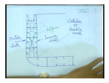
So, these are the aspects one we will have to see. In any guess in double wall what is happening? The moment I go for double wall construction obviously, it is entirely the longitudinally stiffened.
