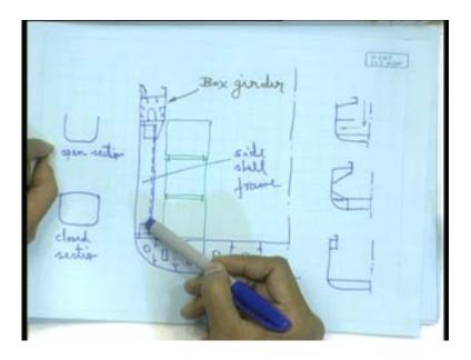
So, this provides you a sufficient strength towards torsion as well as longitudinal; obviously, as well as longitudinal, but this alone is a I mean much less stiffening would have been required if we would have calculated only on the basis of longitudinal bending; bending longitudinal strength, but this is provided to provide called additional torsional strength as well as your side shell stiffening.
