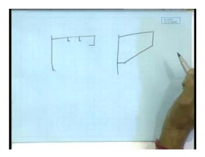
Say general cargo ship once again, you have the deck opening. So, stiffening of this was done by means of a hatch side girder and then stiffening of the deck you had those deck longitudinals etcetera.
