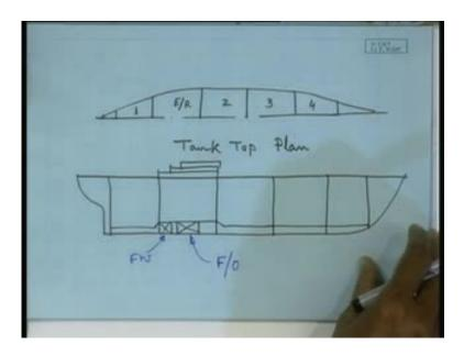
While continuing in double bottom you may see what I have drawn here in this. Suppose, this one is your fresh water and say this is my fuel oil. We can see that there is a gap in between, I have kept a gap in between, so this - the arrangement is, I mean, it could have been as well say you have the well let me so it is a little exaggerated
