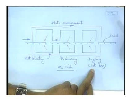
So, to protect it from that corrosive environment there are different schemes, one of the scheme is painting it with some kind of anti corrosive paint etcetera, but that will be done when the product is complete. Means, when you complete the hall before delivery you give the final coat of paint, but till that time what happens you have to also protect it because, otherwise it will lie in the open atmosphere, whatever expose to the atmosphere will corrode.
