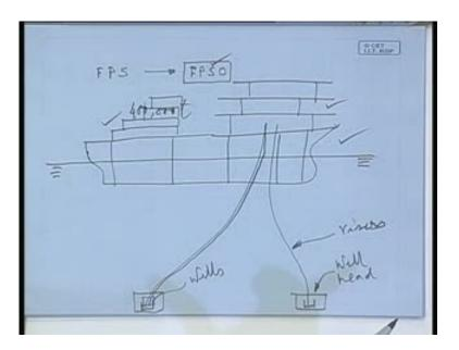
So, FPSOs are, essentially, floating vessels, ships; what many people are doing - instead of building a new vessel, they are converting the oil tankers, converting the huge tankers, because they are very huge; oil tankers are very huge - of the capacity of, the biggest tankers were built or around 400,000 tons dead weight - roughly half a million ton
