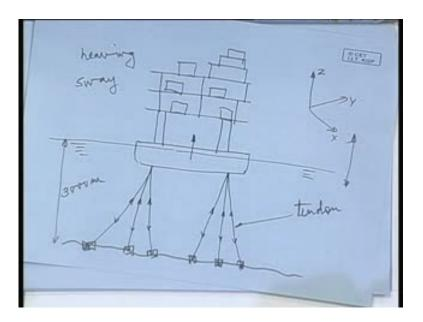
So that is what is essentially the tension leg platforms. The technology as of today - that it can go down up to almost 3000 meter water depth, it can be installed in such deep offshore oils for production of this, what do you call, crude; here the biggest challenge as such is, fixing the bottom seabed connections.
