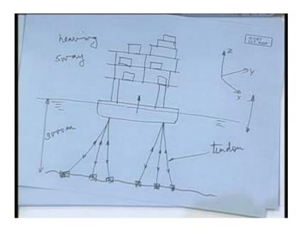
What is happening in this tension leg platform is - this platform is a floating structure; means that entire super structure - the super structure is called the decks, various decks will be there over which you will have accommodation also, you have all kinds of machineries and what not. It will be a very heavily equipped, sort of, place and this will be supported on some kind of floating submersible, some body which is floating.
