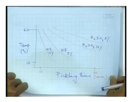
So monitoring of that continuously with time; so you will have to have a proper process developed such that as it monitors the concentration is falling from 10 to say it will gradually fall. It is not a step function, it will gradually fall so accordingly, gradually you will have as it is falling you will have to increase the pickling time.
