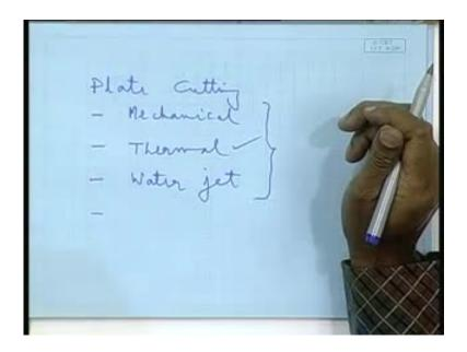
What all types of methods can be used? One is obviously a mechanical cutting, this is a mechanical cutting here, remind you, we are talking about cutting steel plates, aluminum plates such material and of the dimension of 10 meter long plates. So, mechanical cutting obviously it is not question of cutting using an axe or a power saw definitely it is not there; mechanical cutting means by shearing we will talk about that.
