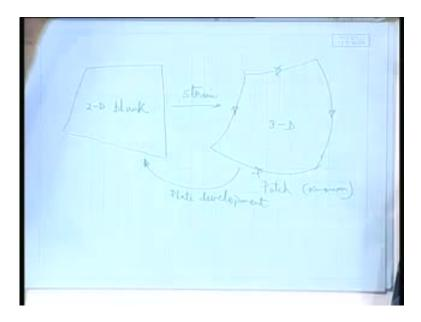
That is what we say that if there is a double curvature in it, like roughly I have tried to draw here, it is curved in this plane, also curved in this plane, so whenever you have a double curve plate that also has the same problem of it, becomes a non-Gaussian curvature. It cannot be developed easily; developed means developed two dimensions, so this is what I have to go for a plate development process.
