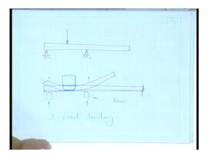
Let us take the case of frame bending, which is simpler, so frame bending means what? Basically frame, it can be thought of as a beam, if I have some such configuration and apply a force, so it bends. That means two supports; one support I am applying a force, so the same thing from this simple configuration. I can think of a machine where in which can be a schematically represented like this (Refer Slide Time: 05:03).
