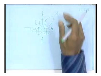
It is not much of a problem - bilge plate, suppose this is my bilge plate - bilge plate is generally is of a radius of curvature that means what? A part of a cylinder, so bending of such things is easy, is done by passing the plate through roller. In the first stage, we have passed plate through rollers to straighten it, now we are passing it through rollers to bend it. So, there will be difference in the roller arrangement, now it will be like this.
