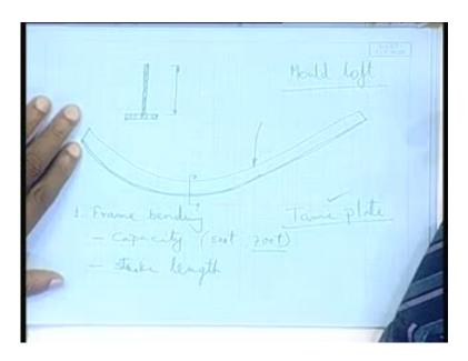
So if that can be done properly, then you do away with the tame plate business, one great unproductive work is reduced (()). It has limitations, but many can be done, because one of the advantage in ship building is the curves are generally of very gentle curve, very high radius of curvature, not very sharp curves - it do not have.
