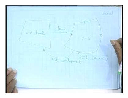
But here, it is little more complicated to get that. You will have to apply the strength and then get the 3-D patch. So, we will see how mechanically it is done and subsequently how thermally it is done.
