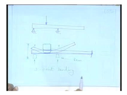
Stroke length is that determines this side RAMs, how much it can move? To what extent it can move? Because, when it is bending, it will go a certain extent, how much? That again limits the curvature. What radius of curvature can be achieved? Anyway, so these are basically two things; the capacity and the stroke length. So that is what in very simple term a frame bending machine.
