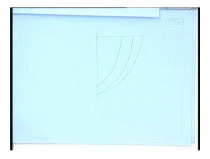
This is curvature, if you cut the water planes with a horizontal plane along the depth, there is a curvature. The frame planes are the vertical sections, they are essentially y z planes, the vertical sections and they are the y z plane that means the section here. Whatever x z plane - any way that means basically the frame planes, so they are coming like this, so it is curved in this plane and curved in the horizontal plane also; the plate is doubly curved.
