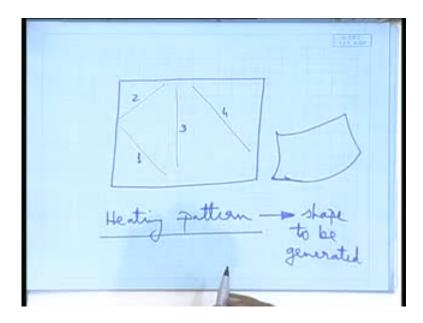
So, heating pattern, so, essentially what we need is that, that we will have to correlate that how much heat is to be, how much heat generates what kind of deformation? Second - what should be the pattern of heating, such that, I get the desired shape? In the first case, it was simple that I have just applied heat and the plate bent like this, a v kind of shape came.
