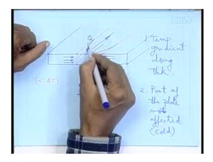
That if this is my case, that means there is no temperature gradient across the thickness, then it transverse shrinkage only will take place.
