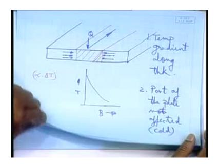
So, the component of that alpha delta T in all these, this thing will be different. Alpha delta T into the length, that length is changing, that is number 1, and because of that, what will happen? The compressive stresses that, that will develop will also be of varying magnitude. Compressive stresses will be of varying magnitude. As you go down from the top surface to the bottom, because at the surface, the heat flow was maximum, bottom it was gradually decreasing.
