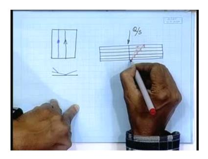
I am drawing it little thicker along the thickness there is a temperature gradient. If it is there, let us assume that the plate is made up of various, I mean made up of various thin layers, or in other words, we consider the plate, we discretize the plate thickness in several thin layers, and we said that if the plate was thin, I could have attained the same temperature both of the surface and the bottom.
