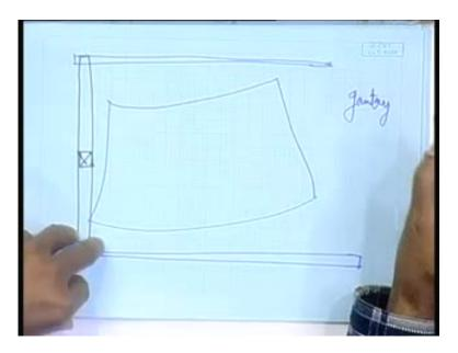
So, same thing, in this gantry, I hang a heating torch which can move in whatever direction you describe to move, it will go on moving and go on heating it. So, thereby I can generate there shape. Now, once that is generated, you move the thing away, move it out; means here you have the along the rails, suppose this is moving, this have the both side rails are there and you have moved it out. This is my heating gantry.
