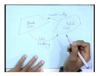
So, there we need to essentially establish the heating pattern such that it conforms to the desired patch. So, how it is done? Once again the same thing like, suppose, well, I mean some arbitrarily I am drawing, say this is my blank, this is the patch.
