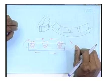
In case of frame bending, what is done is - you have the, suppose the frame, a longitudinal, this is my neutral axis, so, take a v shaped zone and heat it along this, say in this beam three such zones along these lines, they are heated means, these are, this I am drawing as the heating lines.
