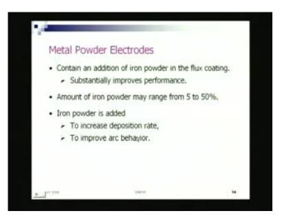
So, before starting going over through gas metal arc welding, let us take a look. And We have seen these three types of electrodes; three types of electrodes for manual metal arc welding or shielded metal arc welding. They are the cellulosic electrode, rutile electrode and basic electrode, and we have another fourth type which are referred to as metal powder electrode. This will be a worthwhile to look into this.
