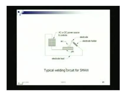
So, this is a very simple schematic of the thing. So, as you can see the power is supplied at the tip of the, I mean power flows through the entire electrode. Unlike in other welding processes, there the power is given right at the tip of the electrode as near as possible, but here, it is given right at the end of the electrode. So, over the entire electrode, the power flows. So, if it get stuck, the whole electrode will get heated up.
