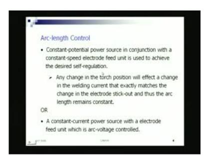
So, any change in the torch position will effect a change in the welding current. That exactly matches the change in the electrode stick out. Electrode stick out is this length, this particular length; that means length from the tip of the nozzle from where, the electrode is coming out and to the electrode tip where you have the arc. So, this length, this is the electrode stick out length, so, it exactly matches the change in the electrode stick out and thus the arc length remains constant.
