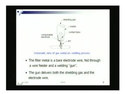
That gas gets ionized. So, what gases, gas you are giving that will determine the, determine the, property of the ionized column. That will determine how much heat is generated or that will have a effect on the heat generated, and thereby, you will have a effect of melting rate, fusion rate, fusion depth, penetrating power. So, that is what it is. So, the, here, the filler metal essentially is a bare electrode wire in the shielded metal arc welding; it was a coated electrode.
