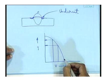
So, where a more precise control of the size of molten pool is required as in out-ofposition welding root passes of varying root gap. A flatter volt ampere curve is desirable. What is that flatter? It is essentially more nearer to constant voltage type. Here, what is happening in a flatter? It is a steep characteristics.
