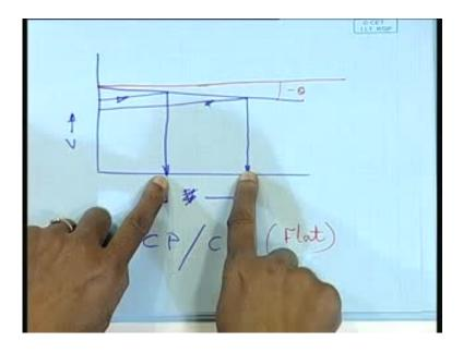
Anyway, so, obviously to have self-regulation, you need to have a flat characteristics, because thereby, as the arc length changes, it gets regularized by a surge in the current because surge in the current can be will be available from a this C P power.
