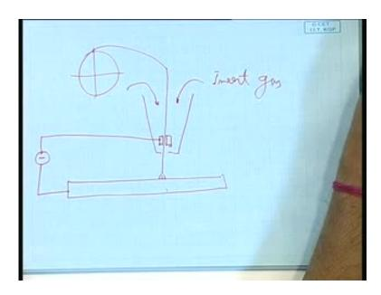
So, essentially, it is like this. So, your power is connected here to the contact tube another terminal to the job and a continuous electrode is fed in, and through the nozzle, you give the so called inert gas. This inert gas provides you the necessary shielding as well as this inert gas acts for the plasma column.
