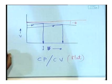
Basically, regulation of what of the arc length, why arc length because arc length corelates to the arc current, which co-relates to the depositional rate because I need required, because at the end of the day, welding means one of the aspect you need is required deposition. Required metal deposition should take place. So, here, what is done? Constant potential power source in conjunction with a constant speed electrode feeding it is used.
