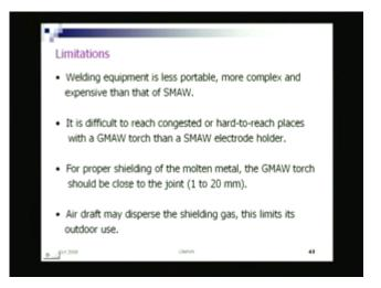
These are some of the limitations. One of the main limitation is external welding becomes difficult outside welding because of outdoor use, because of dispersion. The wind may disturb. Well, so that is all with gas metal arc welding. Next, we will look into possibly gas tungsten arc welding.
