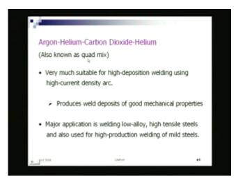
There is something called Argon-Helium-Carbon dioxide-Helium, it is a quad mix. That means argon and helium is mixed, carbon dioxide and helium is mixed, either both are mixed. So, it is very much suitable for high-deposition welding using high-current density arc for high deposition. What happens is with helium, the heat quantum increases because it has a higher, what we call that ionization potential. So, it contributes to heat additionally.
