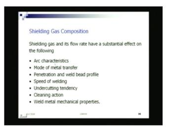
Shielding gas composition, it has a substantial effect on this following arc characteristic, mode of metal transfer, penetration and weld bead profile, speed of welding, cleaning action, mechanical properties, all these even the gas composition it matters.
