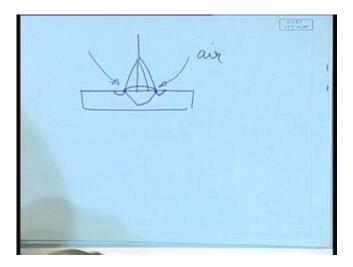
So, the fission zones becomes wider. This is speed of the arc increases as the arc length is high. Arc length is high means, essentially the arc voltage is high, and also may lead to
