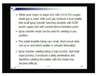
Well, here we see that argon and argon rich with 0.5 to 5 percent oxygen shielding gas, they are generally used. That means, if I use argon or argon oxygen shielding, then we attain a, I mean we can, one can attain so-called spray transfer mode with such gas mix mixture. A true spatter free spray transfer becomes possible with direct current electrode positive supply above the transition current. That means, in globular transfer, you have
