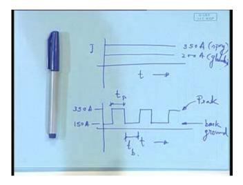
So, I can set this power supply in such a fashion that each pulse will detach one droplet. So, number of pulse I know how many droplets. So, I can control my deposition very precisely. I set the speed of the welding machine. That means speed of the movement of the torch that I know. In 1 second, it will travel so many centimetres or so many millimetres, whatever and also I know that in 1 second, how much, how many droplets it will deposit. I have an idea of the droplets.
