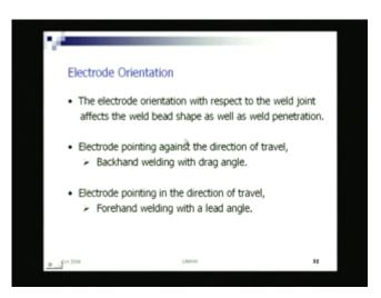
Electrode orientation as I was saying, the electrode orientation with respect to the weld joint, that also affects the shape of the weld bead. That also affects electrode pointing against the direction of travel is backhand welding. It is referred to as backhand welding. With drag angle electrode pointing in the direction is called forehand welding with a lead angle.
