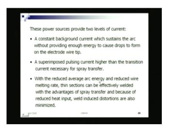
So, what happens is heating. That means, extra heat is going in this case, but here I am controlling. So, whenever there is no metal melting of detachment is taking place, the current is also low, the heat input is also low. So, in this type of wave form what we can see that the overall, we see that the average heat going in to that average arc energy. Thereby, the average heat going in to the metal plate is less. So, what it results in to welding to these distortions is also minimized.
