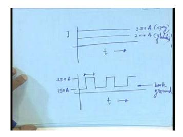
In pulsed, what will happen is, it would be something like this. That means, this is 350 because at 350, I am achieving desired spray transfer. So, I make the pulses of 350 and then, I bring it down. So, depending on the number of pulses, I am giving per unit time. So, many droplets will go. This pulse size is such; this is the microsecond size, whatever is such that in this one pulse, one droplet goes out.
