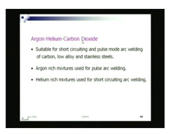
If it is argon, helium, carbon dioxide, well this is good for welding of low alloy and stainless steels, low alloy steels otherwise, and stainless steels. Argon rich mixtures used for pulsed arc welding, helium rich mixture for short circuiting arc welding.
