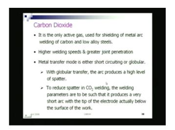
So, here we will take quick look. Carbon dioxide is the only active gas, used for shielding of metal arc welding gas metal arc. It produces globular transfer, produces a high level of spatter. So, there are techniques that it produce a very, I mean welding parameters should be such that you have a short arc.
