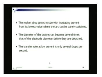
So, the molten drop grows in size with the increasing current from its lowest value, when the arc can be barely sustained. So, what is happening is the molten with increasing current, it grows its size from a lowest value when the arc can be barely sustained. The diameter of the droplet can become several times than the diameter of the electrode, which I have already said.
