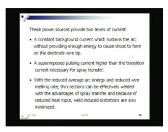
So, this pulse mode, so for pulsing this what we need is a pulse mode power supply. So, these power sources, it provides two levels of current. Constant background current, which sustains the arc or else telling which sustains the arc without providing enough energy to cause drops to form on the electrode wire tip.
