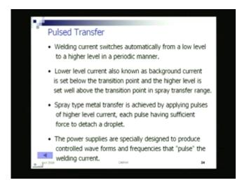
So, that is what low level current also known as. Background current is set below the transition point obviously, and it is set below the transition point and the higher level. That means, this higher level pulsed current is set well above the transfer transition point in the spray transfer range. So, the transition current could be somewhere in between.
