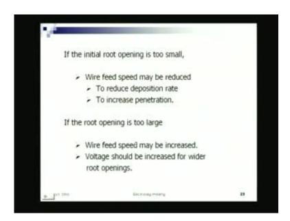
No, the whole process is such that we cannot go for a very high speed welding. Had it been a high speed welding, the case would have been different, it would have opened up, it would have a opened up, but here is a the very process is such that we cannot have a very high speed welding. So, here, necessarily the shrinkage is in this direction that means it closes. So, accordingly you take proper precaution.
