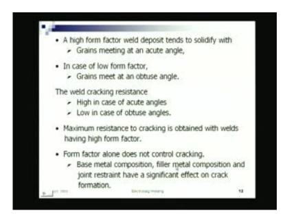
Well, so, that is one aspect also it does not mean that only form factor alone controls the cracking, definitely not. So base metal composition, filler metal composition, joint restrains, all those other aspects are there, but what it means is this is one of the important aspect, the form factor which needs to be controlled, such that I have a higher value of it, such that I achieve a higher resistance to cracking.
