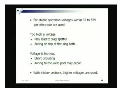
Well, with thicker sections higher voltages are used that means, higher means not this too high, it is not that like we have given a somewhat a range 32 to 55, it means when you weld the comparatively on the thinner side, you use lesser voltage; when you go for the higher thickness, you go for the higher voltage, but well, if you weld 400 meter thick plates possibly much higher voltages will be needed that we are not talking about here.
