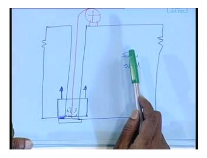
So, what are the features? As you can see the features are it is a vertical position welding, there is the first and fore most as we have seen is a vertical like submerged arc welding is only down hand welding, whereas, gas metal arc or shielded metal arc welding there are all position welding. Here, electro slag is only vertical welding; you cannot do it in a horizontal mode, down hand mode, neither you can do it in a overhead mode, so, only vertical.
