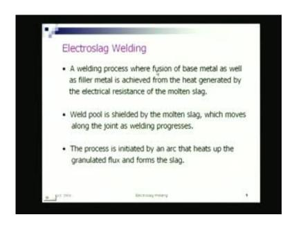
Here, it is the Joule heating or the resistance heating of the molten slag that is how, so, this is the fundamental difference. In electro slag welding, the heat source is from the molten slag, the Joule heating of the molten slag. So, what do you see that, it is a fusion welding process definitely; here the fusion is achieved from the heat generated by the electrical resistance of the molten slag, here and the weld pool, as you can see in this schematic.
