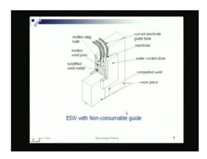
So, small amounts of flux are added at an interval to compensate for the consumption, or in other words, the flux consumption is very nominal. So, these are schematic of the process.
