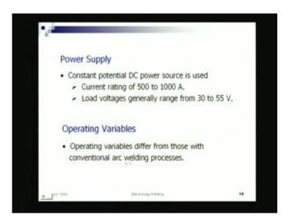
This method can be used to weld sections of virtually unlimited thickness, any thickness can be welded. Well, other features are power supply here; generally you use a constant potential DC power source current ranging from 500 to 1000 ampere. Load this voltages generally arc voltage essentially 30 to 35 volt and the operating variables differ from those of conventional welding processes.
