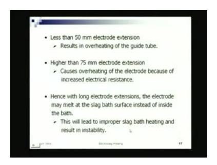
So, this will lead to improper slag bath heating and result, well, hence, long so lead to improper bath heating and result in stability.
