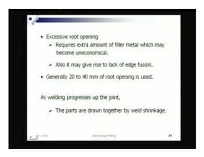
Here, what you are referring as welding progresses up the joint, the parts are drawn together by weld shrinkage. That is there, that possibility is there, as the weld progresses, it is drawn together, that, it tends to close, but because of the other rigidity, that does not create a problem, but if we just two individual plates without any restraint in it, if I try to weld, it will gradually close, then you would not be able to weld it.
