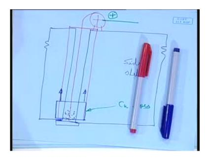
The process is repeated till completion. As the welding current is carried by the guide tube, it needs to be insulated. Required insulation may be provided by flux coating on the outer surface, fiberglass sleeve or insulating tape. This is a complicated business, because that consumable guide - consumable guide means what? The guide which is supporting the feeder electrode, and the guide tube also it is providing a support but it also gets melted and deposited.
