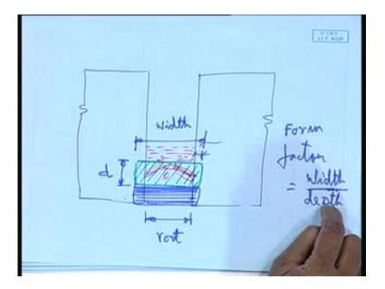
So, what I need? I need a high form factor because the weld cracking resistance is high in case of acute angles, and a high form factor gives an acute angle. What is high form factor? Higher width, lesser depth, that means I should be able to maintain a lesser depth of weld pool, that means it is preferable to have a wider root gap preferable to have a wider root gap, such that I can make this width to depth ratio higher.
