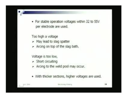
For stable operation, voltage is within 32 to 55 volt per electrode is used. You can see the voltage level. For any other welding, the your welding arc voltage vary within the range
