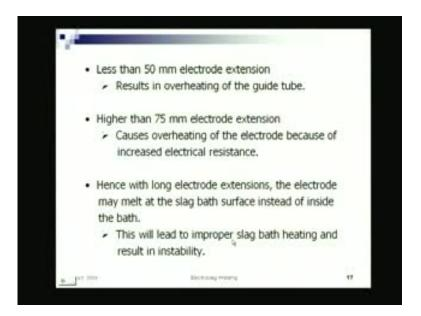
Less than 50 millimeter results in over heating of the guide tube; higher than 75 causes over heating of the electrode because of increase electric resistance, that same thing what we used in case of gas metal arc welding or even submerged arc welding is more the length of extension, more heat is generated there because of the resistance of that part squared the current.
