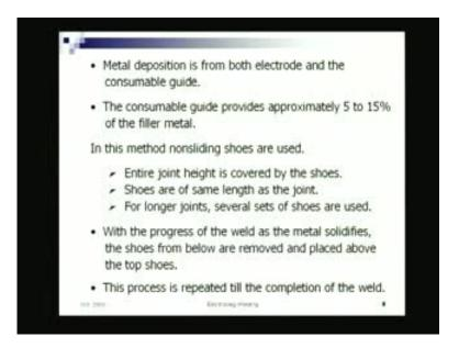
So, here we have talked about metal deposition, I mean when you use a consumable guide - consumable guide means what? The guide tube also gets consumed means also gets melted and deposited. So, that is what it says that the deposition is from both electrode as well as the guide. Here, it provides additional 5 to 15 percent of filler metal.
