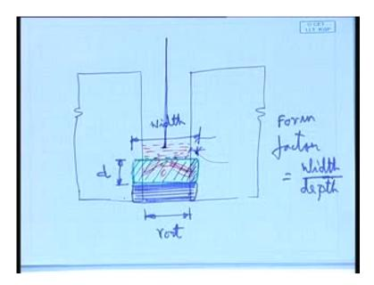
Leads to poor circulation of the cooler slag at the bottom, because you see, the slag at the bottom is somewhat cooler compared to the slag at the top. So, still some kind of circulation is needed. If the circulation is not there, the slag will get solidified below.
