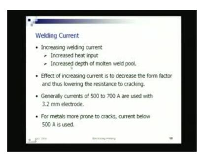
So, that is what, because if I increase the welding current, it will increase the depth of the molten weld pool. This depth increasing means form factor reducing, but we do not want to reduce the form factor, it has to be kept as high as possible. So, the welding current is kept lower. That is how we see the effect of increasing current is to decrease the form factor and thus lowering the resistance to cracking.
