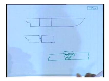
So, once started it continues to completion, a single pass welding process irrespective of plate thickness. What does that mean that means? It can virtually weld any thickness of plate at one go in a single pass with whole process is like that. In other conventional welding processes, say you are welding in a down hand position; a butt welding you are doing to flat plates; you are welding, you have a edge preparation like this.
