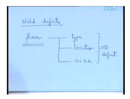
But when you are actually doing a fabrication work, you cannot cut out a sample; so, you will have to have a means of Non-Destructive Testing which is also refer to as NDT, right? So, well, let us first look in to the type of defects. What are the types of weld defects? Now, this is what defect? Because, what happens, the welding is such a process, it is really very difficult to ensure that it can be a, a welded joint can be 100 percent defect free, right?
