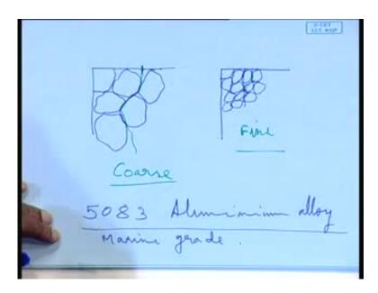
That is, it is referred to as 5083 Aluminum alloy, this is a this is of marine grade. By marine grade, you mean, they are used in marine environment, right? This 5000 series alloy, they are they have a high magnesium percentage, high magnesium content of the order of 4 and a half percent magnesium which provides for the corrosion resistance in marine environment, this particular aluminum alloy.
