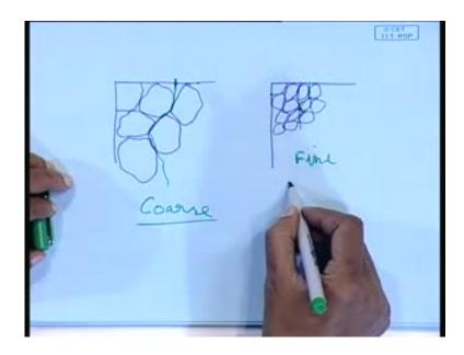
Why that is happening? Because of your grain refinement; I mean, without going much detail into the metallurgical aspects, certain simple simple rules are like this. That means, if the grain is refined means, the grain size becomes smaller, you have higher strength; if the grain sizes are bigger, you have lesser strength, right? Little bit if you see, suppose these are two samples, now say, these are my grains as we can see in the in a powerful optical microscope.
