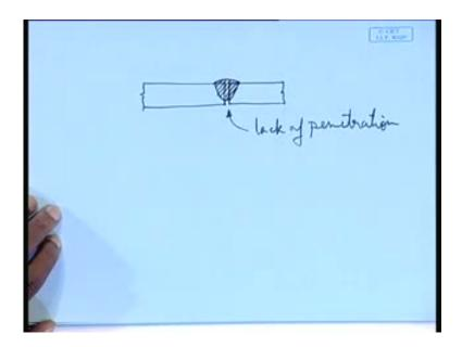
Lack of deposition: this may happen because of improper weld parameter like higher welding speed, less melting rate of the electrode as lead to improper deposition proper, full deposition has been taken place, that is, lack of deposition.
