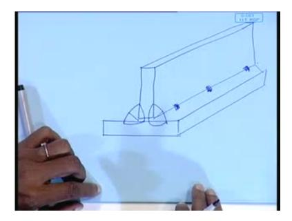
I was telling you probably in the previous class, just a simple case of fillet welding we had been doing, right? So, with a submerged arc, the fillet was like this; both sides fillet, right? And, and a crack was observed in, right? In the center line, through and through crack from the surface; still inside, through and through crack took place.
