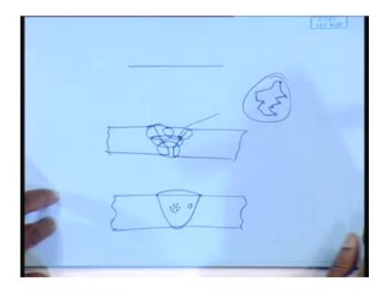
Then, you have slag inclusion means, when you do a multi, multi-run welding, suppose, with a manual metal arc welding with a multi-run, means, one run you have given, then whatever slag was there you have removed it; you have given a second run, a third run and so on. Every run you are giving, you are removing the slag; if you do not remove, it meticulously a small speck of slag may remain inside. Suppose a slag has
