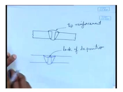
Then, lack of penetration: lack of penetration is, that is, say again, suppose a butt weld is being done, right? And, the fusion zone looks like this; that means, deposited metal did not penetrate through the thickness, did not penetrate through the thickness, and there is a lack of penetration at the root root. Deposition has been taken place, this is a lack of
