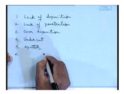
Then, that will tell us whether that flaw is a defect or not; if it is a defect, remedial action has to be taken, right? So, that is how. So, let us see now, what are the so called defects one may observe in case of fusion welding. We will talk about the ones which are more, well, I mean, so called mostly observed and which are more, which has a predominant effect on the performance of the structure.
