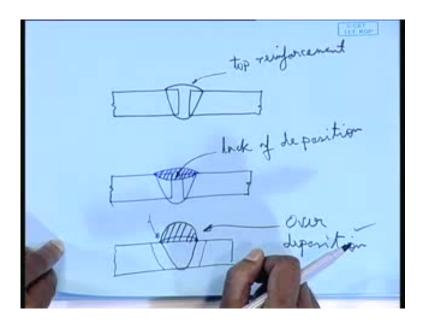
Similarly, here it is more serious lack of penetration, because, this part will act as a gross discontinuity in the structure, will behave like a crack as if... So, there will be a much greatest stress concentration, lack of penetration is more sever defect than lack of deposition, right? So, this is what lack of penetration is.
