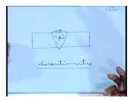
So, as I was saying, the flaws depending on type location and size, well as far as the location is concerned, as we can see, this is a, say, a welding has been done. Now, a flaw can be at the surface, a flaw can be somewhere here on the upper surface of the joint, can be at the lower surface of the joint, can be at the bottom, can be at the middle; different location in different orientation, right?
