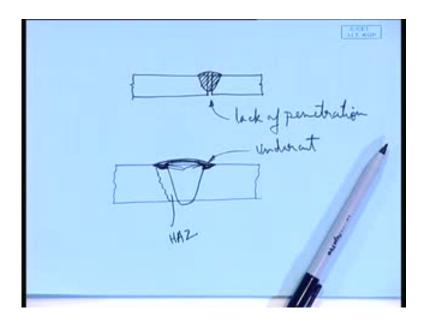
So, that is also not, I mean, that is not desirable, so, over deposition can also be taken as a defect. What is to be done? Lack of deposition, if it differs; what is to be done? Well, simple; you will have to deposit additional layer; you will have to re-weld it, simple; to get the proper deposition here, what is to be done? You have to grind it, you have to use a grinder, cut it off, right? So, that is what is over deposition.
