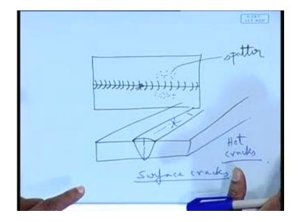
Then, spatter spatter is a thing, you see it is not a directly itself, is not a defect; say, this is my weld line, right? This is my weld line, that means, along this, the welding has been done, say a butt joint has been done; a butt welding, that means, two flat plates have been welded, and you see in some location, there are lots of such small small droplets of metal droplets are there, this is what is refer to as spatter.
