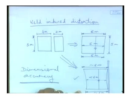
So, any thermal operations done, like we have seen in thermal cutting, oxyacetylene cutting, when we do, also, it may lead to deformations. Similarly, when we do welding also, it would lead to deformations, which can be termed as Weld induced deformations or distortions, Weld-induced distortions; because, you see, the fundamental requirement or the desirable requirement of welding is, as we said that it is a process to join two
