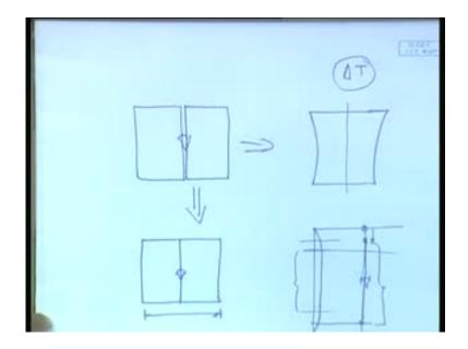
Why it is becoming like this and not a straight line? That means, when these two plates are being welded, we say that the final shape is becoming like this, right? And not, well just straight lines; that means, the overall breadth has become less, but not uniform. What what is happening? It is Essentially, what happens is, say over the length, it will come straight, again it will taper down. This is how the shrinkage takes place; that means, over a certain length, it will be all uniform.
