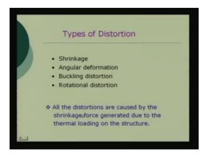
So, we see, because of this, essentially, because of this non-uniform heating and cooling cycle as well as non-uniform expansion and contraction, final thing what is happening is development of shrinkage forces, development of shrinkage forces. That is why it is said that all distortions, these distortions are related to weld induced distortions or thermal distortions.
