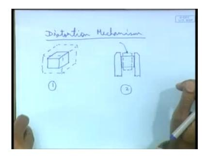
So, it is like this. Supposingly, we take a say a small piece of, say a small piece of steel cube, a cube of steel, right? And, we subject it to uniform heating, uniform heating. So, what will happen? In the hot state, if you can measure it, we will find that the dimension has increased, right? It has become somewhat like this.
