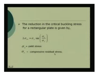
So, that is why you will see a stiffened panel is made. It is more prone to buckling in fact, right? The compressive stresses degrade the buckling strength. What happens, the compressive stress residual stresses, it reduces the buckling stress. It is actually through some such, some sense it goes that the reduction of the critical buckling stress for a
