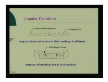
The stiffener is held in a position by means of supports; it is not allowed to move this way that way, stiffener is held in position, but the free edge of the plate is the edge of the plate is free, so, it deforms; that is what is here, it has it it is it is lifting up, deforming, right? Both the edges, they had just as I am welding, the plate is lifting up, right? That is because of the fillet welding and this is because of the in in case of butt welding.
