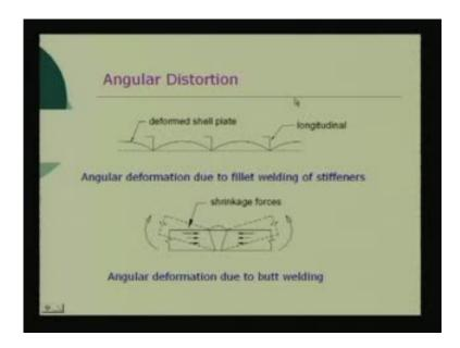
Then comes angular deformation, right? Angular deformation is outer plane deformation; that means, it is going out of the plane of the plate. So, what do we see? Here, two simple diagrams are given; these angular deformation due to fillet welding of the stiffeners, angular deformation due to fillet welding of stiffeners.
