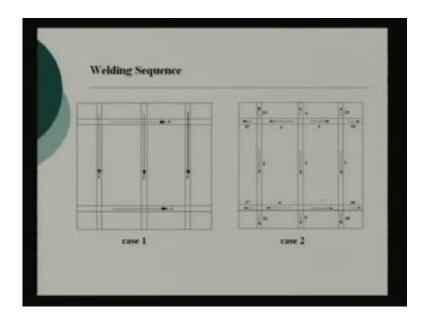
See, these are very simple technique but have to be done, I mean in a proper logical fashion. Depending on the size of the structure number of lugs, the dimension of the lugs, welded, heat it up, and then, weld it. When it is cools down, automatically it is putting in tension. So, one side first I weld it, other side only I heat up and weld. So, these are the distortion mitigation techniques. Well, in the next class, little bit we will see in the welding sequence.
