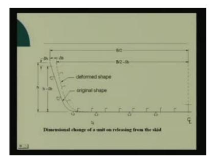
So, we have seen, say here, I mean how the distortion, they effect. Here, it is a sketch of a, say a bottom shell, a bottom part of the of a ship structure, just the double bottom unit. A section if we look into, here you have the bottom shell which is stiffened by longitudinals and the part of the bilge plate, and well, a part of the side shell if I say so, but you can consider it to be a small unit, one part of the double bottom, and here. you
