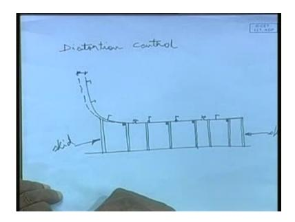
So, essentially, solution is suitable shrinkage allowance that means, here, you provide suitable shrinkage allowance. Whatever shrinkage is taking place, such that, this height short fall in height is taken care of. As well as this sinking whatever is taking place, that has to be, that means, you will have to provide the allowance, such that, it is actually done like this such that, after shrinkage, it will shrink back to the design designed dimension.
