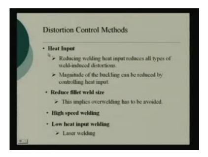
So, you can see the heat generation is much much higher. So, more heat does not mean that more distortion; it is the rate of heat input. That is what actual influences extent of distortion. So, that is how this controlling heat input, controlling distortion through controlling heat input is essentially controlling means, essentially selecting a welding process where the rate of heat input is reduced by increasing the welding speed.
