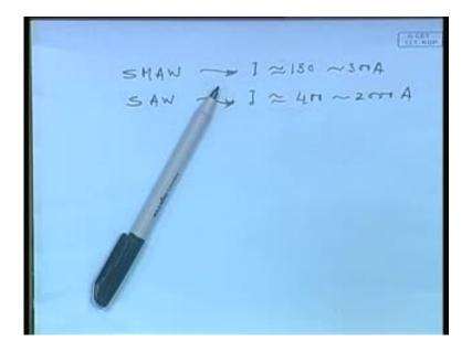
Why because if you see submerged arc welding, sorry, this shielded metal arc welding which is a manual process. Here the current level would be of the order of, say, well, around 150 to about 300 amperes. Whereas, as we have discussed in submerged arc welding, the current level could be, say around from 400 to, say 2000 ampere.
