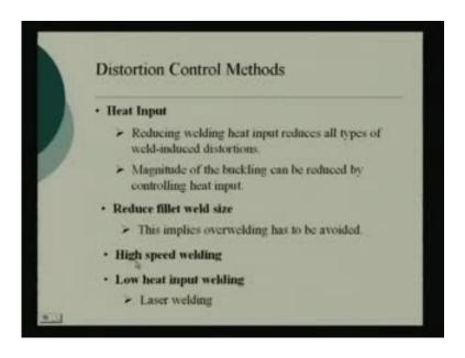
So, that is another aspect. Next is high speed welding. We have already talked about in connection with heat input because high speed welding, well, obviously, in conjunction with the heat input, this gives us mechanism for controlling the distortion. That same thing can be talked about given a name as low heat input welding. As you can see the
