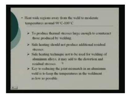
So, here, some of the details of that process is I have mentioned that the heat wide ranges away from the weld to moderate temperature of 90 to 100 degree centigrade that means, that way the heat temperature level is kept much below to produce thermal stresses large enough to contract these those produced by welding. That is the whole idea is to contract the stresses which may form by the welding.
