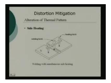
So, these are some of the methods of so called distortion mitigation. So, here, one example, so, it lies on the fact of alternation of the thermal pattern. Distortion is due to a certain thermal pattern. Now, if I alter the thermal pattern to our advantage, such that distortion is reduced, so, that becomes a method of distortion mitigation. So, one of the method is side heating.
