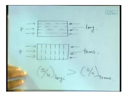
If it is stiffened in this direction, identical plate is stiffened in this direction, so that the top one longitudinally framed and bottom line is transversely framed, isn't it. This has been done by longitudinal framing system, as if this is transverse framing system, both of them are under compressive load in this direction.
