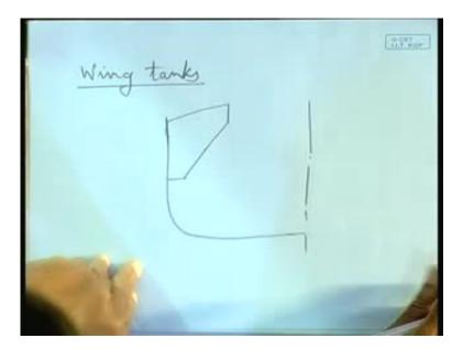
Wing tank, as you can see, the name, it is kind of a tank. As if right this wing tank and that the tank is in the wing that is how the name of the wing tank. In bulk carrier, we will see, we have already when talking about the different type's vessel, we have seen there is a kind of vessel, which is referred to as bulk carrier.
