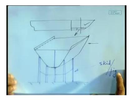
A framing system based on the longitudinal framing system; so that is what I mean - whole this so called concept of the double bottom construction, these are the 3 d units fabricated from the stiffened panels.
