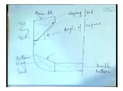
The solution would be that cut of that space, provided a plate cut of this space and also provide a plate. That means now when I load cargo, the cargo comes like this. When I unload also the whole things gets unloaded, because this slope of course, I am drawing it very shallow. We will have a definite slope - required slope such that the cargo will come down automatically to the central part, from where it is pumped out or through grab, it is taken out.
