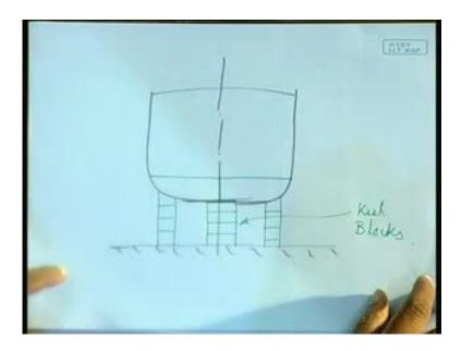
When a ship actually is put on what you call on the keel blocks, when the ship is under construction. You cannot really put it on the floor, is not it. Then, it will be difficult to work. So, it should have a proper base over which it can be put. So, if this is my floor line that means the ground line, the ship sits on such blocks. These are blocks, generally you have three rows of blocks to support, over it sits and they are referred to as keel blocks.
