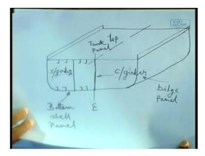
These are the side girders; obviously, you will have in the floor such cuts, which are referred to as what you call the scallops, so this whole thing would look something like this, a double bottom unit. So, this double bottom unit is manufactured from or fabricated from this plating, this stiffened panel. The stiffened panel is the tank top panel, then you have the bottom shell panel, this is my - we have talked about - even you can have the bilge panel.
