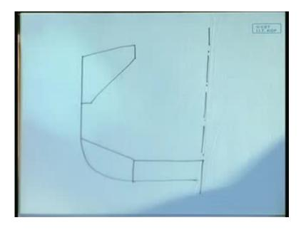
There is a kind of vessel, which is referring to as bulk carrier. It carries cargo in bulk, well let us take a look at the sectional view of a bulk carrier, wherein we have the concept of wing tank; this is what the wing tank is.
