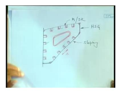
Then now for local strengthening, because of this particular plate, these dimensions can be substantial. So, they may get buckled in between, because of others loads coming on that.
