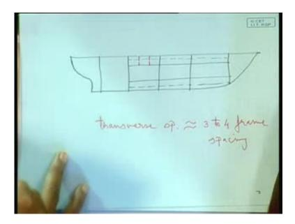
It could be one of these, it could be these and the longitudinals will run like this, isn't it. So, again you need to provide necessary support such that the span does not become too much, because otherwise your supports are at the bulkheads.
