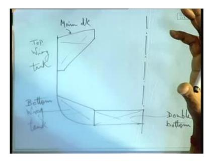
This side girder you assume in this case, as if the double bottom as ended in the side girder. This side girder is also water tight, such that this is a separate tank in that case. Similarly, here also I can see some tank like space, so this is referred to as bottom wing tank and this is top wing tank. This is a typical feature of bulk carriers only, in bulk carries, you have such wing tanks, why this wing tanks are coming?
