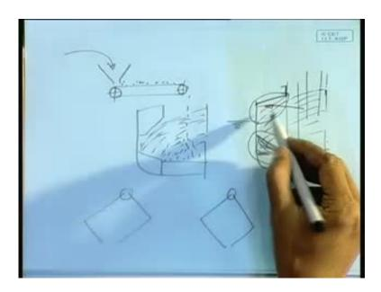
These plates are referred to as sloping bulkheads, sloping bulkhead of top wing tank, sloping bulkhead of bottom wing tank, so I get a tanked space. So, these are my wing tanks, what is the purpose of this tank? Tanked these spaces, same as that of your double bottom space; that means, otherwise, what was happening is, as it is we could not use this phase, so by making a tank, it does not mean that I will carry extra cargo there.
