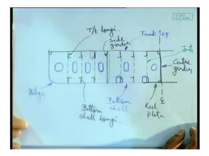
It only is said that - where longitudinal is difficult, where it becomes difficult? Where you have interference with the cargo, mainly which is the main cause of concern at times, when I have to shift from this to transverse framing system. Otherwise, all longitudinal - that is why in oil tanker, the entire framing arrangement is longitudinal framing arrangement. So, double bottom also is similarly will go for totally.
