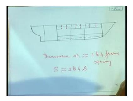
If transverse spacing is represented by capital S, it is 3 to 4 times the small s. Here, you will have the transverses, how? That means at intervals like this, you will have the transverses - wing tank transverses; they will be refer to as wing tank transverses.
