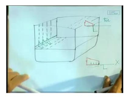
Just to show how the things that they take ship? Say, this double bottom has been fabricated and then what happens? The other stiffened panels or the side shell panels we have talked about - so side shell panels, once they are fabricated, they are erected here that means you have the double bottom.
