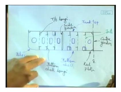
Well, there is one more word about these girders. The center girder is generally a water type girder, totally water type plate. Means, this center girder divides the entire double bottom, in port and start boat independent tanks.
