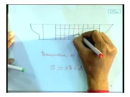
When you see this, when you talk about this transverses, right at intervals, so in the same interval, you will have a web front in the side shell, a bottom wing tank transverse or a plate floor, top wing tank transverse web frame, bottom wing tank transverse plate floor. So, such will be the deployment of the transverses or the transverse stiffening members.
