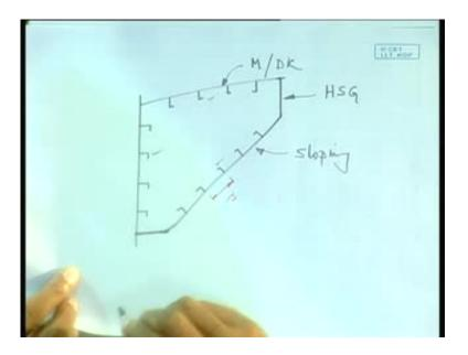
The questions of transverses come that means transverse, so the spacing of transverse spacing is generally how much? It is generally 3 to 4 times the frame spacing or in another words, the span of the longitudinal remains 3 to 4 times its spacing. Frame spacing - frame spacing is spacing of the longitudinal, this is my frame spacing.
