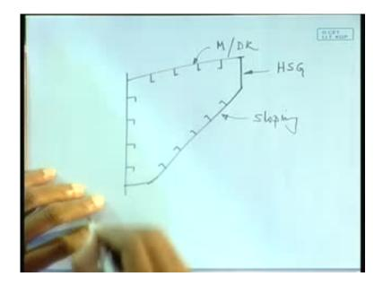
That means, I have additional space in addition to the double bottom, I have bottom wing tank, I have top wing tank, they can be utilized. Now, if I just look into the top wing tank or the wing tanks, the construction point of view, it is like this. This is the main deck, this is my sloping bulkhead and then this can be the hatch side girder. So, deck is longitudinally stiffened, once again we are using longitudinal stiffening of the deck.
