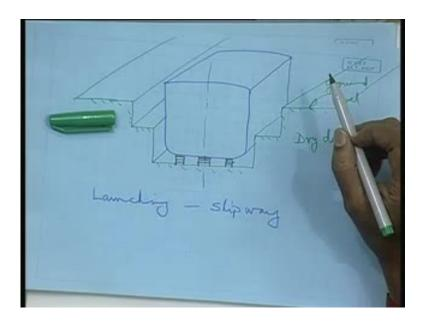
Best is, you built it in the dry dock. So, what do you do? In the dry dock, the dock is dry, means the gate is closed. Here, the rows of keel blocks led, depending on your handling capacity, either you start installing the subassemblies here. Generally minimum thing installed is the units, means that say with the double bottom you start and then bring the side shell erect. If I have more handling capacity, this entire block is fabricated in the shock floor; from there it is transported here.
