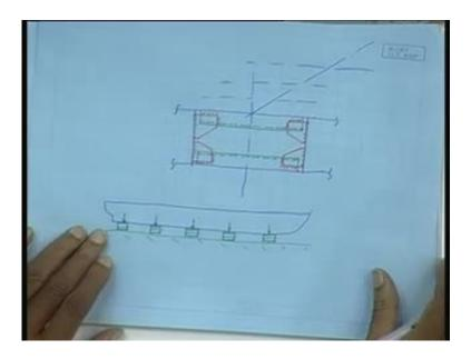
This is a dry dock, where it will sit over this keel blocks. The load on this comes - so, you can see the entire load of the vessel, will be supported only at the certain points. Sort of 3 rows of blocks - I mean 3 columns of blocks and certain number of rows, there will be some sufficient gap between them. The entire weights of the vessel are supported in these points, so naturally the structure has to be very strong.
