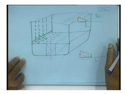
Duct keel arrangement is nothing but, it is forming a duct. This space as you can see, is forming a clean duct, this is running all along the length of the ship, isn' it? It will be to some extent in this fashion, as you have applied to show it here. They are the two side girders running along the length of the vessel; it is only in one box.
