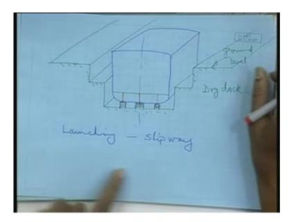
How this keel blocks will be led? That also will depend on - I mean, if you see inside what is the construction, you will have to have, where the keel works have to be spaced,
