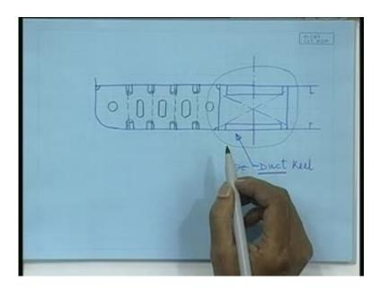
We are showing here. These two are water tight side girders, so this space becomes a protected closed duct. What are the great significances or great use of this arrangement? Well, one definitely provides a much better support for the ship structure; we had been talking about putting the ship on keel blocks.
