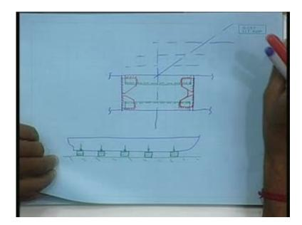
Again, what happens? Your bearing area becomes less. Suppose your depth of this is 200 and if I keep 100 millimeter gap, then this becomes only 100. So, support area becomes less. So, has to be some optimum, generally 50 to 75 millimeter is kept, they are the simple logic. So that is how this duct keels. Here, this entire thing - taken this entire construction, is referred to as duct keel, because it forms a duct.
