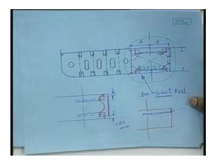
That is also one aspects of the stiffening member; that means to support the load, so that is how. What we see is the duct keels, the function here. Here, as we see that the connections are with brackets, so one can have this is the simplest way of doing it. That means you have four separate brackets, so the alignment problem is not there at all or it can be converted into one piece like this. This is just one piece of - also it can be converted like that.
