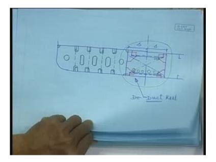
Because, then what happens? The entire plate is supported here and I am providing at every frame space. Only thing to provide is the proper load path, you will have to put the brackets like this, with this side girder, now it is bracketed; so brackets are provided. There is no more need for longitudinal - this longitudinal is not there, this construction is like this or a cleaner version - let me draw, I will show you.
