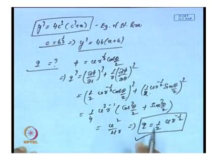
So, from which we can easily get y square is equal to four c square into c square plus x, because we have taken phi is equal to constant as given us the stream lines. So, c is equal to constant this is again gives us a stream line equation of stream line, so that why this can represent a flow. Now, if I take c is equal to b to the power half, but we have seen is called y square is equal to 4 b into x plus b.
