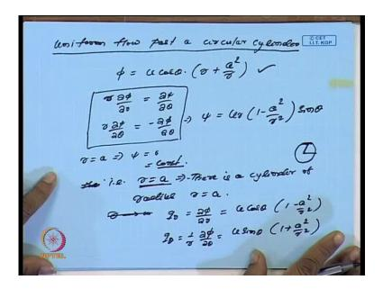
Now let us come to that uniform flow past a circular cylinder. This is where one of the interesting problem, which is many times has a very important role, when it is. Suppose I consider the velocity potential pi is equal to u cos theta into r plus a square by r. Now if I apply question, and suppose we have given this pi, but, what will happen to this flow here, if I have this is the pi. Then we have to find what is string function, and to find the
