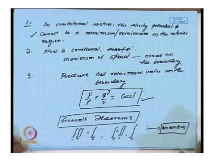
In irrotational motion, the velocity potential phi, cannot be a maximum, or a minimum. It cannot act an, cannot be a maximum or minimum in the interior region. The second one, when the motion itself when flow is a rotational, now a large in the contest of fluid flow
