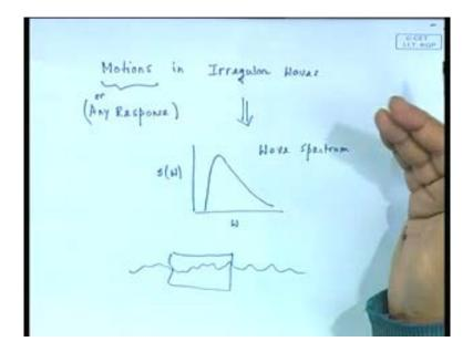
See today, we are going to talk about motions or ship motion. Let me just just write motions actually. Although, we are calling motions, it could be any response. What I mean is this. See, we have seen in the past lectures that irregular waves can be finally represented by means of a wave spectrum and this is nothing, but a sum of regular waves. So, I know my environment that, have talked in last two lectures.
