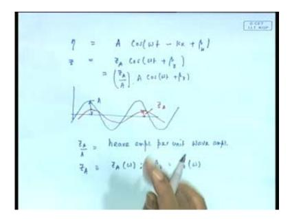
So, I will take a sample as heave motion. Now, see let say I have a wave, particular wave one frequency wave eta one or say, well I will put that one later on. So, it is given by a cos omega t minus k x. Let us put it this way or even I can put a beta if I want.
