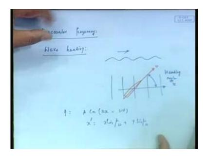
See, remember we are now putting our ship in a regular wave field not a random wave field, we have a single sin wave coming, let say a wave which is going like that, in this direction, so if I were to draw the quest line, the quest line will look like that, going this side x axis, but the ship need not be travelling this line it can always travel along this, it it can travel any direction.
