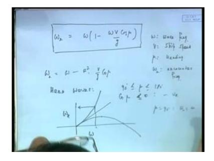
We end up getting omega e as omega 1 minus omega V cos mu by g, when I am writing this omega is wave frequency V is ship speed mu is heading, and so this is the form now, but look at this equation, this equation is quadratic equation in omega in other words, basically omega is becomes omega minus omega square into V by g cos mu.
