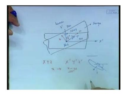
So, I have now here one system use colours X dash, Y dash, Z dash some point O here and this is hypothetical shape, but actually the shape would have been somewhere here, and in this case body fix system would look like well may be this is x, this is y, this is z, you understand that means, small x y z is fixed on the body with respect to that you can define your lines plan, your hull surface, etcetera.
