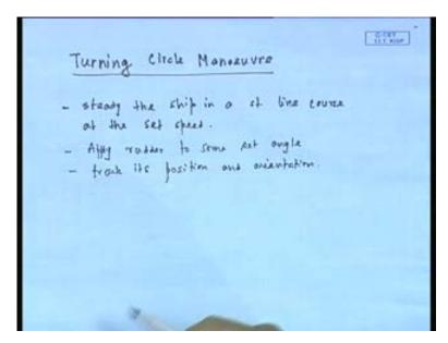
See excuse me, in the last classes, we discussed about pull out manoeuvre, spiral manoeuvre, both of which were used for stability, finding out whether the vessel is stable or not; then we talk of zigzag manoeuvre which basically assessed, how quickly it responded to rudder.
