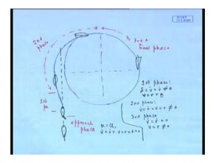
What would happen? Let me just draw this diagram, so the ship is coming here initially you may apply the rudder here, at this point you probably apply rudder, this is my rudder we apply. What would happen you know, you follow the trajectory it turns out the trajectory, may be I should do some other colour, it will go (No audio from 03:52 to 04:11) like that (Refer Slide Time: 03:54) (No audio from 04:12 to 05:03).
