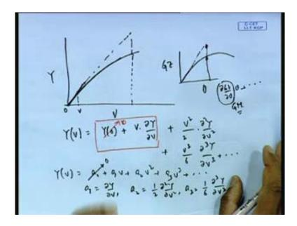
So, if I would have to make a straight line; I would have call G Z what I would have call Z G Z by d theta into theta plus this part is nothing but G M but if I want here I need this, I do not need this; if I have to use G M theta I would have up getting this as G Z. So, the analogy is exactly the same because, at larger value of the force there can be possible non-linear variation it may actually be like this, I need to use higher order coefficients.
