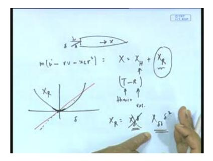
Let us, look at this X force because I need to now know the X force against rudder angle because, when I put the rudder angle delta remember my X force changes means rudder
