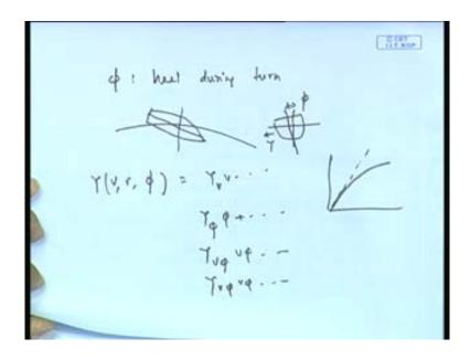
So, if you say cross section it is heeling outward like that, so when its heels my Y force that comes swill depend on the angle of here also suppose, you have two degree heeling there will be some effect of that; so then Y becomes function of v r also phi. So, then I can have this we have seen this v but, v v etcetera then also I can have phi phi etcetera then I can have also have phi phi etcetera then also I can have then I have v phi v phi etcetera then I have got r phi r phi etcetera.
