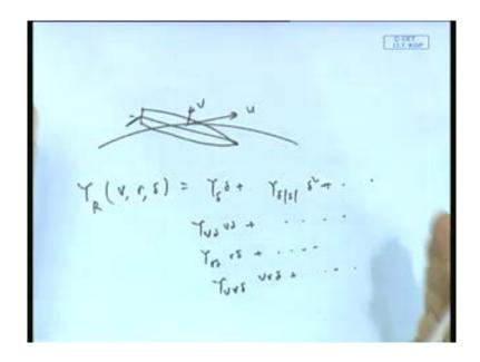
Similar, will be n against delta that is the rudder forces but, there are more twit remember, I am putting the rudder when I am having certain v that means; I am going turning like that with a v. So, I have a u here, I have a v here at that time I am putting this rudder, so my Y rudder force is a function of v, as well as r, as well as delta because after all I am applying the rudder in my simulation when I have already some vary of non zero v non zero r.
