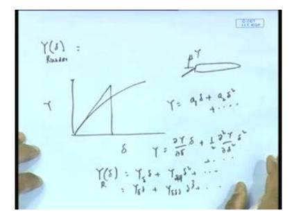
Now, rudder Y at delta that is Y rudder, what we are doing? Delta verses force you know I give the rudder; I want to find this Y force let suppose the graph is like that what is this? This is going to be Y force is going to be again a 1 delta, plus a 2 delta square, plus etcetera if see this would have been d Y by d delta into delta linear term but, I have 1 by 2 d square Y by d delta square into delta square goes like that.
