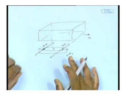
I would have had a, I will come back to this then, a say a carriage here, some kind of a carriage here. Below that I have say two struts, the system. At some point of here, I am attaching my model, this attachment point can be fixed, this full thing is attached to that by some means, along this line I can make the model to go up to and fro horizontally.
