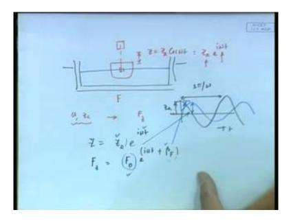
What we do here, this is my tank here, say water tank. So, let us put the water like this, and I have the body here. What I do is that, see I want to give it a particular oscillation motion z, or say z a e i omega t, I am controlling it, omega and z a. I can have a mechanism, some kind of circular mechanism by which I can push it down. Then what I do by an instrument here, I measure the force that is been required to push it down, the force that is coming
