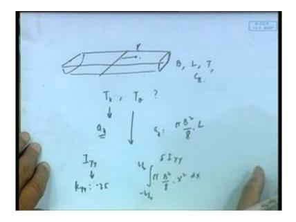
So, here it says I have a wooden log of uniform cross section or let us take a barge, I have a barge here of uniform cross section, which can be any uniform of side B with B length L and it is statistical stable. Now, here once again the question I ask was, what is my T z and T theta? Estimate that. What you see, then I said that use your engineering judgment, I mean I am trying to leave it to you, use your engineering judgment for that, for estimates
