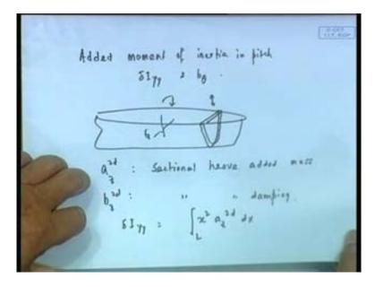
Let me look at this estimate for added moment of inertia in pitch and also the damping, that is basically del I y y and b theta. See just like heave, if I have this ship here, and if I took a section, and if I have my sectional added masses was a z 2 d, was my sectional heave added mass and of course, you can also have that similar damping, I can always call this.
