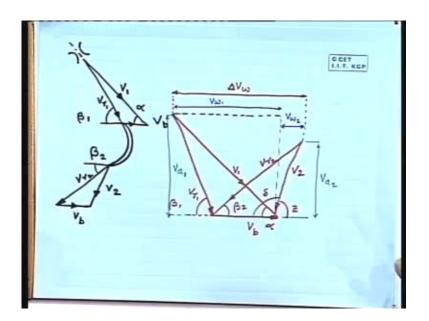
What is  $V_{omega2}$ ? If we see this is  $V_2$ . This angle let us call it any name, let us say it is Z. If we take  $V_2 \cos Z$  then we get  $V_{omega2}$ .  $V_2 \cos Z$ , if we write... this is  $V_2 \cos Z$ .
