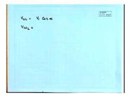
Let us see  $V_{omega1}$ . What is  $V_{omega1}$ ? If we see this,  $V_{omega1}$  is nothing but... If we see  $V_1$  and project it on this plane then we get  $V_{omega1}$  and this angle is alpha. So,  $V_{omega1}$  will be  $V_1$  cos of alpha. Now, let us determine  $V_{omega2}$ .
