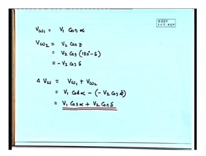
Basically, delta  $V_{omega}$  is equal to  $V_1$  cos alpha plus  $V_2$  cos delta; the way I have drawn the delta. If we draw or if we denote delta in the same manner then we can use this relationship. We can determine also the inlet blade angle.
