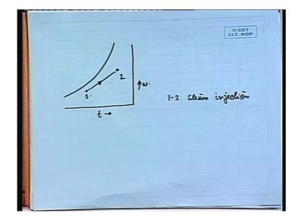
One can have another option also for winter air conditioning. The condition during winter is somewhere here; our comfort condition is somewhere here. One can have steam injection. If you inject steam, then you will increase the moisture content and you will increase the temperature also; here, t and w. This is 1 and 2. 1 to 2 is steam injection. This is also possible.
