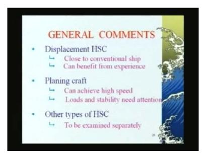
Displacement high speed crafts are generally close to conventional craft going to round bottom boats, and designing this one can benefit from experience- understand that high speed boats which are not displacement type our experience is limited.
