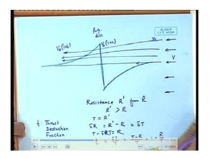
We have increased the velocity. I have made a small sketch which I will have to show you. I have a propeller here. I am drawing the plan. The water was wave forward, far forward of the propeller disc. The water was moving at some velocity V. Let me say or V V a or will speed of advance. Let me for the time being V. This is the propeller disc.
