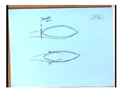
Now, a single cruise ship, this is a single cruise ship; this is the area of the propeller disc. I have draw the plan. So, what we see here? The boundary layer will form there like that and the propeller is inside the boundary layer. It may be partly inside partly outside depending on its diameter.
