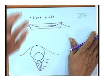
Let, let, me draw it. This is the ship moving with a velocity V forward. How will the wave profile look? Let say it generates transverse waves in such a manner that there is a wave crest at the front and wave crest at the back, and the waves travel this way in the reverse direction because the ship is going forward. What will be the velocity of water particle here? Can you tell anybody? What is the nature of movement of a water particle here? It would be circular.
