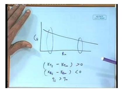
We have seen the ITC line which says or any frictional line for that matter. If I have Reynolds number here and the coefficient here, then it reduces as the Reynolds number reduces. Similar to ship case the propeller model propeller will be somewhere here and ship propeller will be somewhere here. So, you can see there is a change, a lot of change in the coefficient of friction.
