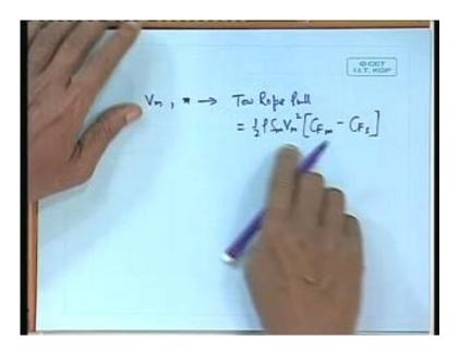
Yes, now I have a carriage I move the carriage as V m and R P m and thrust and torque I measure, but I also apply a tow rope pull equal to half rho S m V m square.
