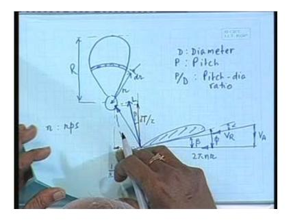
Let us say this is the propeller; this is a rotational axis. We will consider an element which is the best way to consider an element is between radii r and r plus D r from the centre; that means we will consider an element like this. This is r and this is D r and the propeller overall radius this we can call it capital R to distinguish it between an element and the maximum radius. We will consider this element and we will see the thrust and torque generated due to this element.
