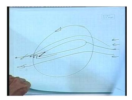
Now, let us see this is the aerofoil section and this is at an angle as you can see. I have already drawn it at an angle to free stream velocity which is horizontal in this direction.
