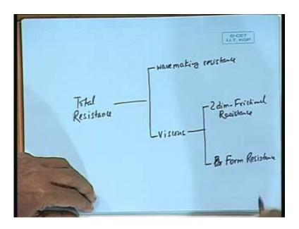
No, it is not like ((build scale)), ((build scale)) is a flat surface, its effect is mainly in frictional resistance. So, flat plate,, unless this one little problem with ((build scale)) if the ((build scale)) is aligned in the in a stream line that would flow pass the ship, then the resistance due to ((build scale)) is only due to two dimensional friction, but if it is not aligned in a stream line the built skill itself may disturb the flow creating separation and eddies.
