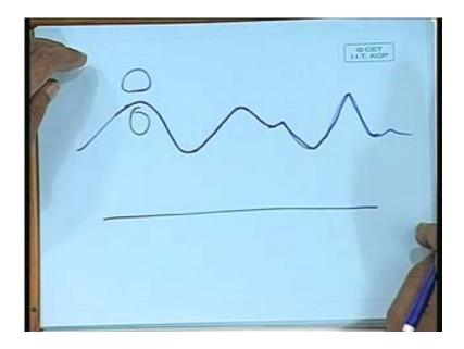
Top of the surface, top surface... Suppose, I have got a wave surface like this, what is the pressure here, here and here, is it constant? No sir. No, then you are in big trouble; it has to be constant and equal to atmospheric pressure.
