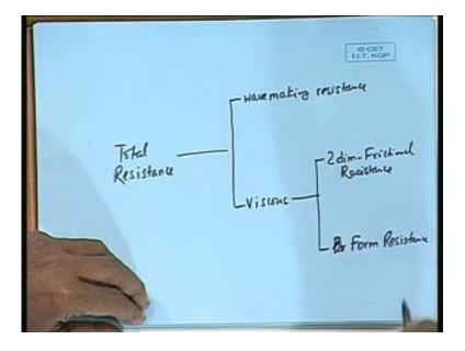
So, in conventional components of resistance analysis we say that total resistance is composed of wave making resistance and viscous resistance, which is two dimensional frictional resistance and form effect form resistance due to form. Normally, this is taken as a percentage of this; so, we have frictional resistance estimate in some manner multiplied by constant, do you understand?
