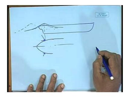
Let us take two cases. What I am saying, suppose you got a wave, which has a stern like, I am not talking about the aft, let us say this stern pressure is high here, so when the body is here, if I draw the body here, the pressure is high here therefore, there is a large component supporting the motion, this component, is that clear?
