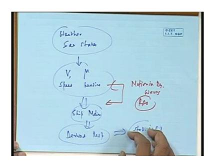
See, you have got various weathers, that are sea states. You have got number of weather a number of weather conditions, you have got number of combinations of speed and heading angle, speed and heading. For all this, you have got ship ship motions.
