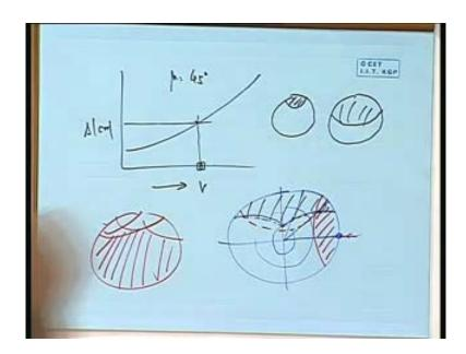
So, what I did is that, simpler case, we shall take, where as velocities diagram are there. Let us say this is like that. Now, I find out that at this angle, at this particular heading, I can go up to all the speeds. No slamming at this angle. I can go up to this much speed beyond that, it is going to slam.
