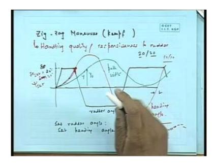
We will start; this part of the lecture also is continuing on ship trials and maneuvers; I will start again from where we ended in last class - zigzag maneuver; now, we understand the maneuver - what we do - we turn the rudder keep on swinging and you measure that; what do you measure? Here at these quantities - this is what I should write down; let me see these terms here or...
