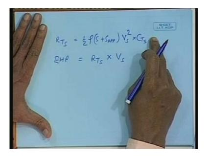
Once you get CTs you can calculate RT as half rho S plus SAPP rho s p a p Vs square for various speeds. And EHP, effective horse power, we have seen will be equal to total ship resistance into (())... -Sorry?- into CTS. And if this is in kilo newtons this will be in kilowatts, this is meters per second, this will be kilowatts.
