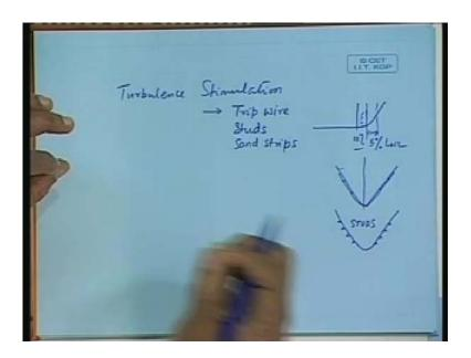
So, use turbulence stimulators. Turbulence has to be stimulated, we have to stimulate turbulence in the fore part of the ship and how do you do it? We have to introduce artificial roughness at the front end of the ship so that the flow becomes turbulent because of existence of rough surface we, as if we are introducing forcible turbulence on the ship fore body.
